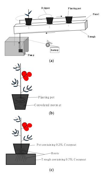
**Figure 1.** (**a**) Recirculating hydroponic system, (**b**) complete root restriction in 1.0–1.5 L pot, and (**c**) Partial root restriction in Cocowool (0.25 L pot + 0.75 L trough).
