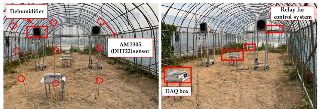
**Figure 8.** Photos showing the experimental setup conditions in the greenhouse (red circles indicate the sensors and red boxes indicate the DAQ and dehumidifier).
