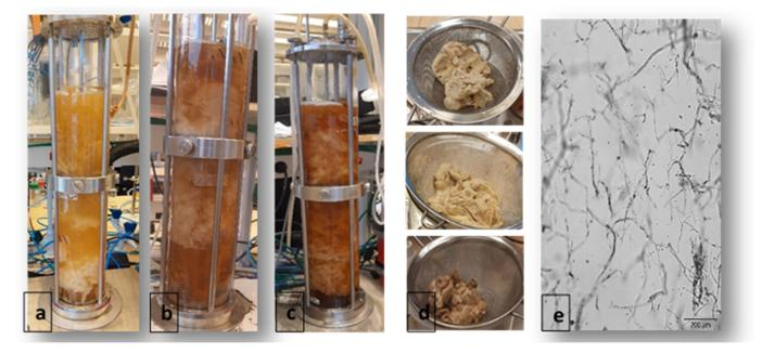
**Figure 3.** (**a**–**c**) Fungal cultivation in bubble column bioreactors using LFCP after the hemicellulase, pectinase, and invertase pretreatments, respectively; (**d**) harvested biomass from the hemicellulase (**top**), pectinase (**middle**), and invertase (**bottom**) pretreatments; (**e**) fungal mycelium obtained after the hemicellulase pretreatment (image was captured by oCelloScope).
