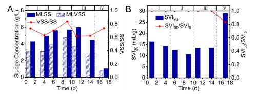
**Figure 2.** Sludge characteristics of SAGS: (**A**) MLSS, MLVSS, and VSS/TSS; (**B**) SVI<sub>30</sub> and SVI<sub>5</sub>/SVI<sub>30</sub>. Period I: 1.8 kg COD/m<sup>3</sup>·d; Period II: 3.6 kg COD/m<sup>3</sup>·d; Period III: 5.4 kg COD/m<sup>3</sup>·d; Period IV: 7.2 kg COD/m<sup>3</sup>·d.
