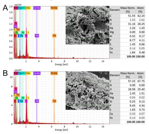
Figure 5. SEM-EDS analysis of the cross section of SAGS (A) Initial; (B) Period III (5.4 kg COD/m<sup>3</sup>·d).
