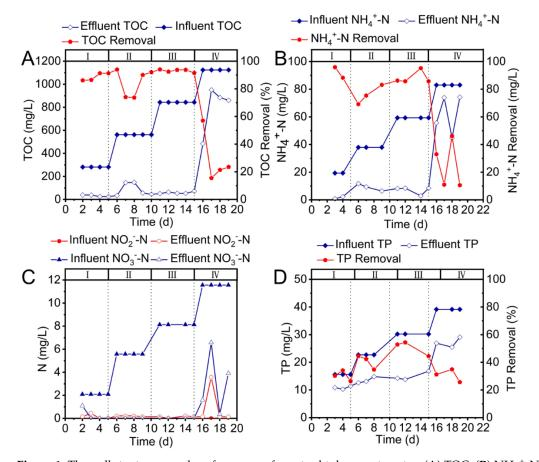
**Figure 1.** The pollutants removal performance of mustard tuber wastewater: (**A**) TOC; (**B**)  $NH_4^+-N$ ; (**C**)  $NO_2^--N$  and  $NO_3^--N$ ; (**D**) TP. Period I: 1.8 kg COD/m<sup>3</sup>·d; Period II: 3.6 kg COD/m<sup>3</sup>·d; Period III: 5.4 kg COD/m<sup>3</sup>·d; Period IV: 7.2 kg COD/m<sup>3</sup>·d.
