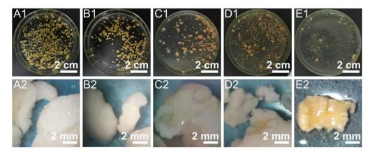
**Figure 3.** SAGS morphology under different OLR: (**A**) Initial; (**B**) Period I (1.8 kg COD/m<sup>3</sup>·d); (**C**) Period II (3.6 kg COD/m<sup>3</sup>·d); (**D**) Period III (5.4 kg COD/m<sup>3</sup>·d); (**E**) Period IV (7.2 kg COD/m<sup>3</sup>·d). (**A1–E1**) were taken by a camera, and (**A2–E2**) were taken by stereoscopic microscope.
