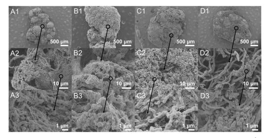
**Figure 4.** The SEM images of SAGS under different OLR: (**A**) Initial; (**B**) Period I (1.8 kg COD/m<sup>3</sup>·d); (**C**) Period II (3.6 kg COD/m<sup>3</sup>·d); (**D**) Period III (5.4 kg COD/m<sup>3</sup>·d).
