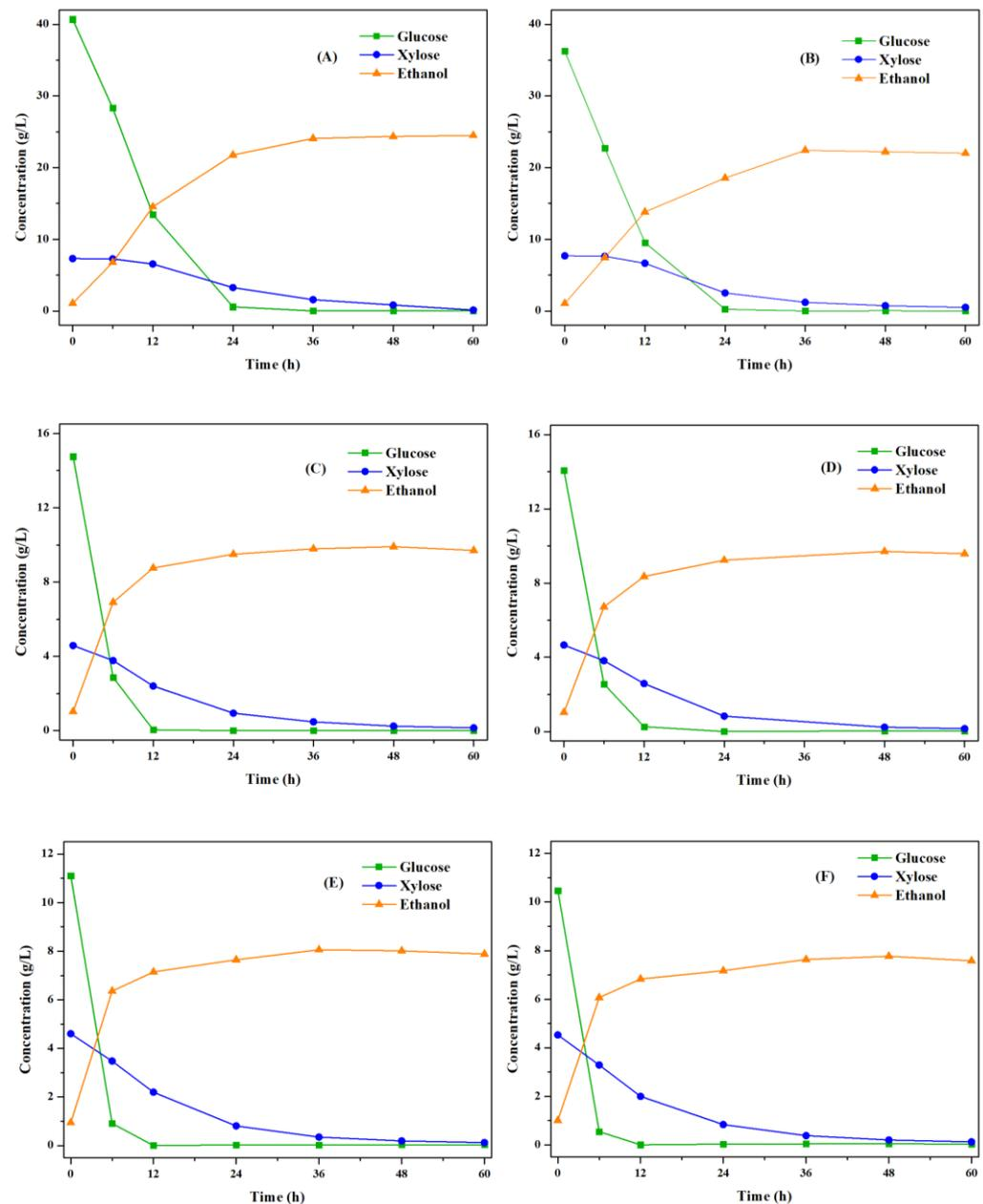
**Figure 9.** Changes in sugar and ethanol contents in the SHF process of pretreated SCB: TEBAC:LA (A), BPP:LA (B), TEBAC:AA (C), BPP:AA (D), TEBAC:LEA (E), and BPP:LEA (F).
