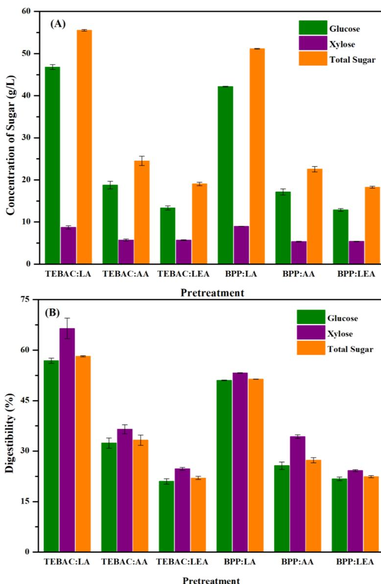
**Figure 8.** The concentration of sugar (A) and digestibility (B) obtained after the enzymatic hydrolysis of SCB pretreated with different DESs at 120 °C and 90 min. As shown in Tables S1 and S2, effects of pretreatment with different HBDS have significant differences statistically (one-way ANOVA, Tukey's test;  $p < 0.05$ ).
