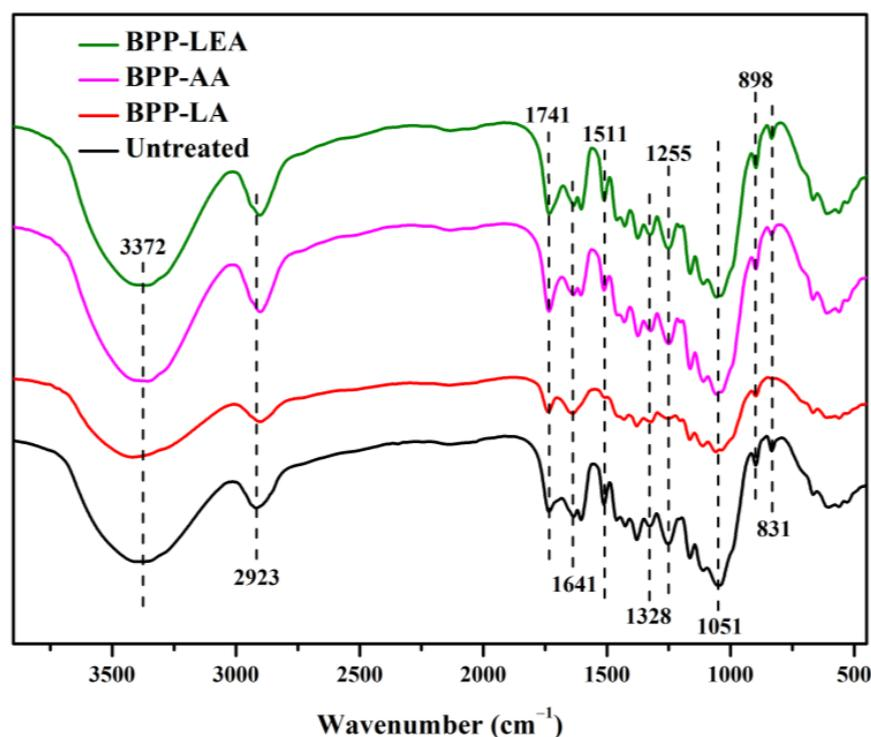
**Figure 5.** FT-IR spectra of the untreated SCB and pretreated SCB: BPP:LA, BPP:AA, and BPP:LEA.
