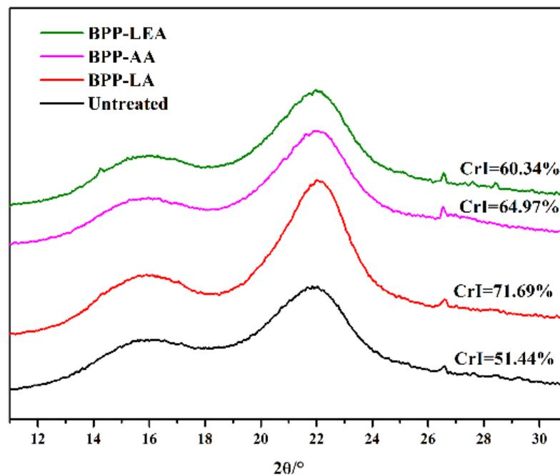
**Figure 7.** XRD diffractograms of the untreated SCB and pretreated SCB: BPP:LA, BPP:AA, and BPP:LEA.
