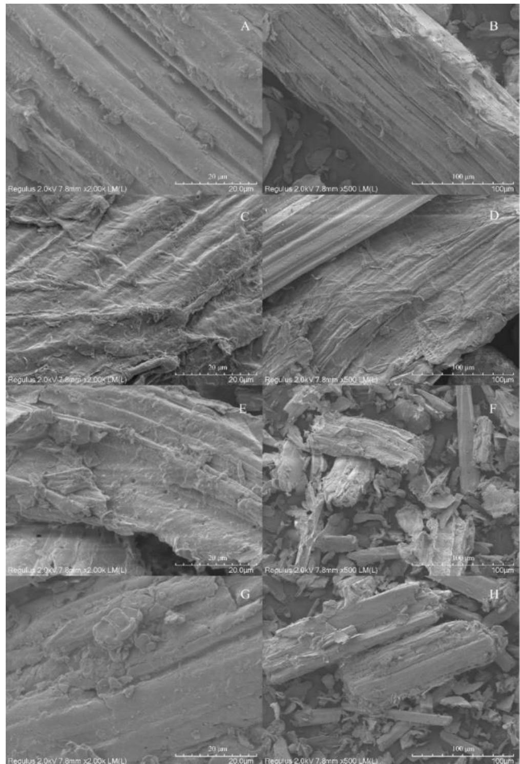
**Figure 3.** SEM images of the untreated (A,B) and pretreated SCBs: BPP:LA (C,D), BPP:AA (E,F), and BPP:LEA (G,H).
