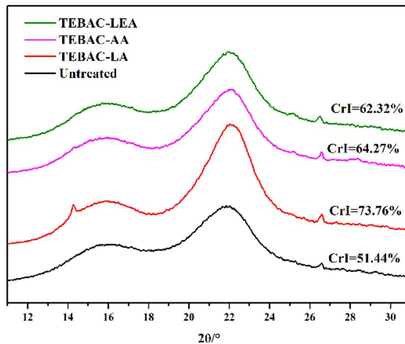
**Figure 6.** XRD diffractograms of the untreated SCB and pretreated SCB: TEBAC:LA, TEBAC:AA, and TEBAC:LEA.
