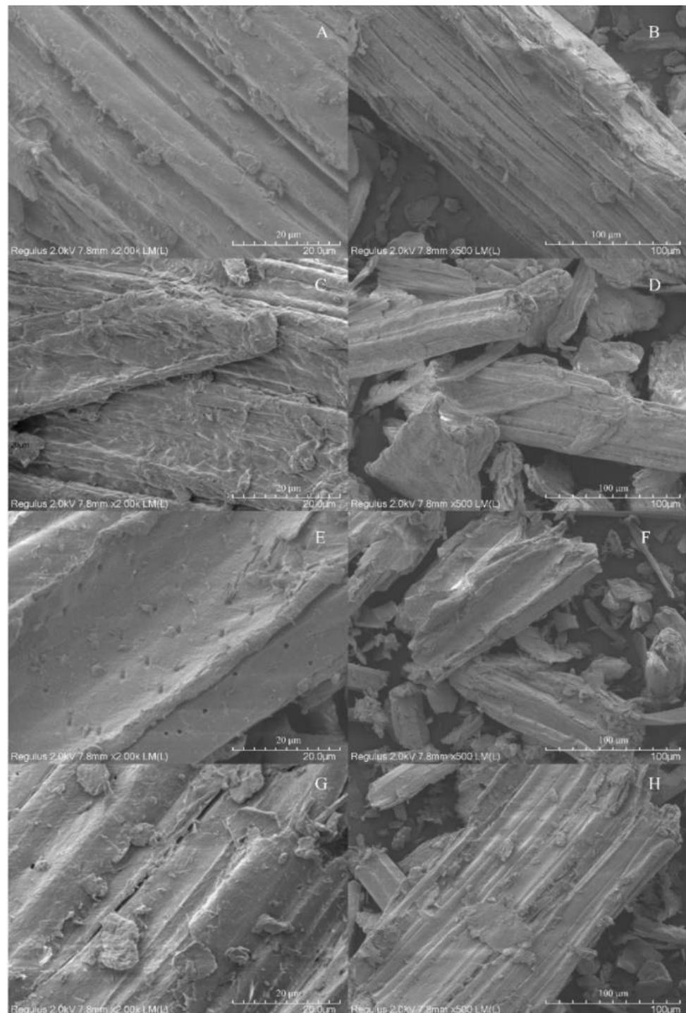
**Figure 2.** SEM images of the untreated (A,B) and pretreated SCBs: TEAC:LA (C,D), TEAC:AA (E,F), and TEAC:LEA (G,H).
