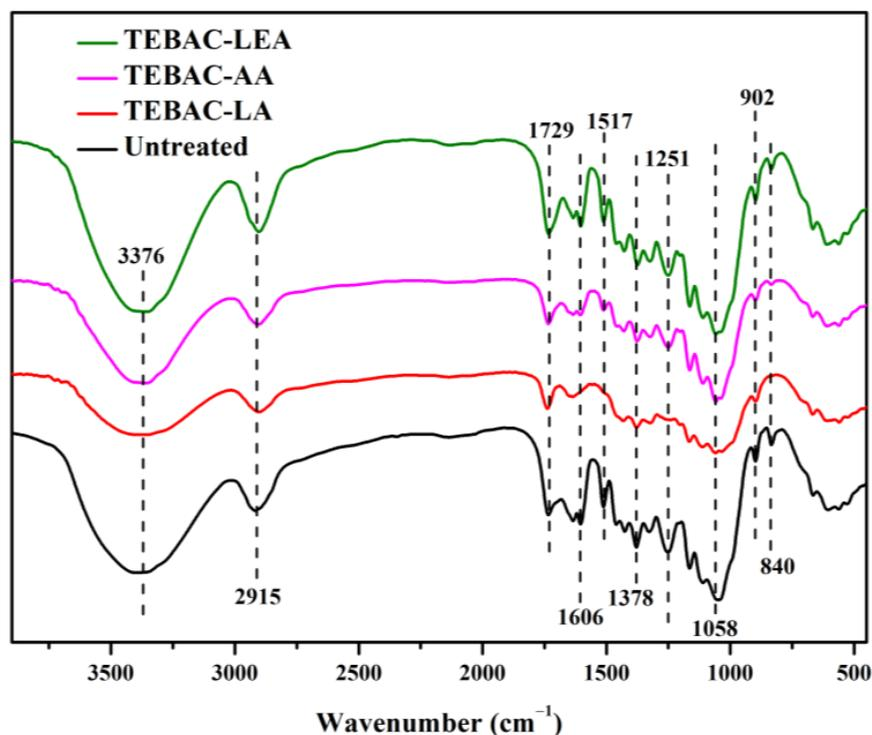
**Figure 4.** FT-IR spectra of the untreated SCB and pretreated SCB: TEBAC:LA, TEBAC:AA, and TEBAC:LEA.
