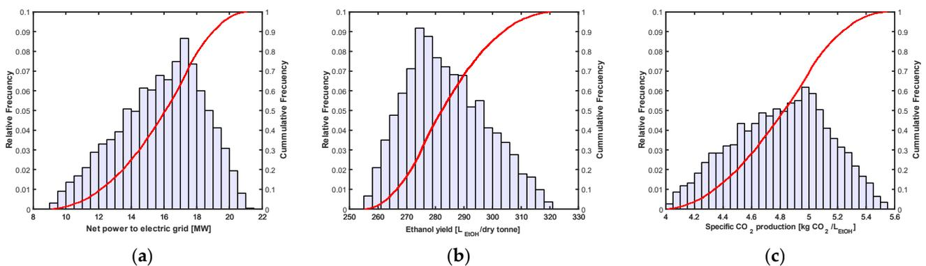
**Figure 3.** Uncertainty analysis results for the net power exported to the electrical grid (a), bioethanol yield (b), and specific CO<sub>2</sub> production (c) using Monte Carlo simulation with 5000 scenarios. Red lines represent the cumulative frequency, while bars represent the relative frequency.
