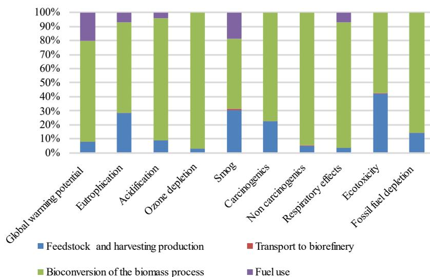
**Figure 2.** Mean contribution of each stage to the environmental impacts of bioethanol production.
