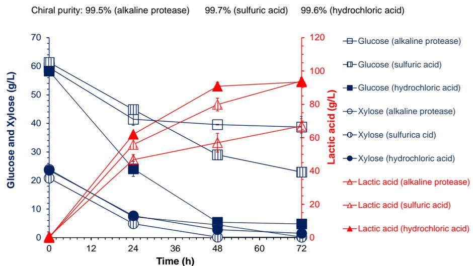
**Figure 2.** L-lactic acid SSCF using cottonseed meal hydrolysate as the complex nutrient source. The cottonseed meal was hydrolyzed by 3% alkaline protease #2, 5% sulfuric acid, or 5% hydrochloric acid. Conditions: 25% (*w/w*)-solids loading; 42 °C, 150 rpm, 72 h. The fermentation pH was controlled at 5.5 by automatically adding a 25% (*w/w*) Ca(OH)<sub>2</sub> solution. Other fermentation nutrients included 2 g/L of diammonium hydrogen citrate and 0.25 g/L of manganous sulfate monohydrate.
