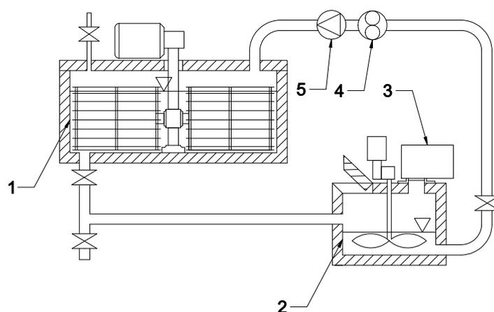
**Figure 5.** Scheme of the research stand. (1) Reactor with a cage mixing system; (2) intermediate tank; (3) microwave generator; (4) mill grinder; (5) displacement pump.
