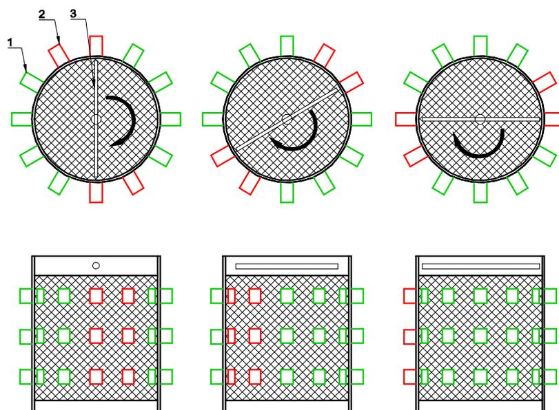
**Figure 4.** Scheme of operation of microwave generators heating the fermentation reactor. 1—green EMR, ON; 2—red EMR, OFF; 3—stirrer.
