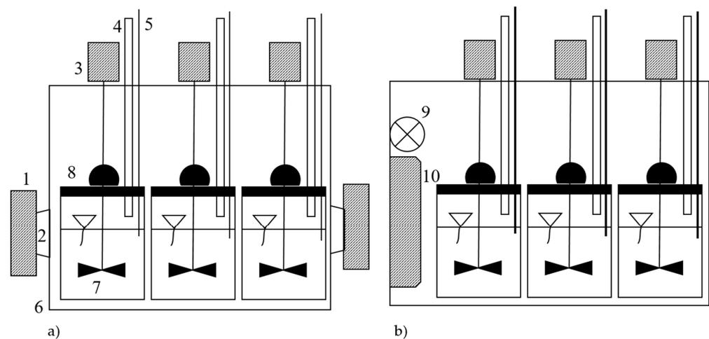
**Figure 1.** Design of experimental stations: (a) microwave heating system (electromagnetic microwave radiation (EMR)); (b) convection heating system (CH) (1—magnetron; 2—wave-guide; 3—agitator drive; 4—pressure measurement and biogas collection; 5—temperature sensor; 6—steel cabinet; 7—agitator; 8—model fermentation tanks; 9—fan; 10—convector).
