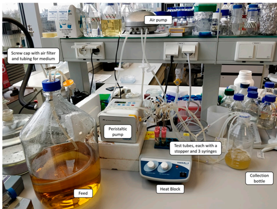
Figure S1. The experimental setup of the ministats. Four 15 mL test tubes are placed in a heat block at 30 °C and are equipped with a stopper and three needles: one for the feed, one for air supply and one for the output. Medium is fed to the test tubes from the 10 L bottle with fresh medium through a peristaltic pump. Air is pumped into the test tube through an air filter, which causes overpressure and the outflow of medium through the output needle into the collection bottle.
