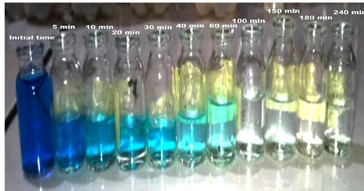
**Figure 1.** Images showing discoloration of indigo carmine solution over time after treatment.
