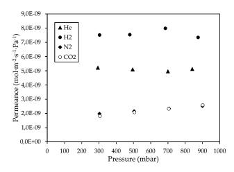
**Figure 3.** Permeance of He, H<sub>2</sub>, N<sub>2</sub>, and CO<sub>2</sub> gases through the CM\_2 membrane at 90 °C, with respect to the pressure.
