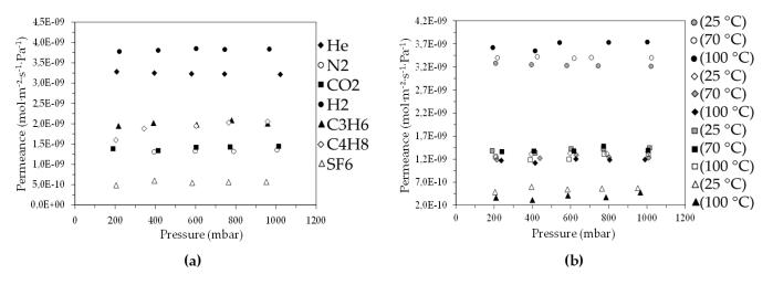
**Figure 7.** Permeance of (**a**) He, N<sub>2</sub>, CO<sub>2</sub>, H<sub>2</sub>, C<sub>3</sub>H<sub>6</sub>, C<sub>4</sub>H<sub>8</sub>, and SF<sub>6</sub> gases at 25 °C and (**b**) He, N<sub>2</sub>, CO<sub>2</sub>, and SF<sub>6</sub> gases at 25, 70, and 100 °C, through the CM4 membrane, as a function of the pressure.
