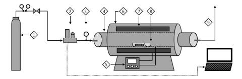
**Figure 1.** Apparatus for conduction of thermolytic processes on supported ionic liquid membranes: (1) gas cylinder (Ar); (2) mass flow controller; (3) pressure gauge; (4) refractory tube; (5) PID temperature controller; (6) tubular furnace; (7) heating zone; (8) ceramic capsule; (9) vent.
