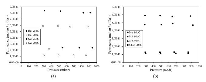
**Figure 5.** Permeance of (**a**) H<sub>2</sub> and N<sub>2</sub> gases at 25 and 90 °C and (**b**) H<sub>2</sub>, He, N<sub>2</sub>, and CO<sub>2</sub> gases at 90 °C, through the CM\_3 membrane, as a function of the pressure.
