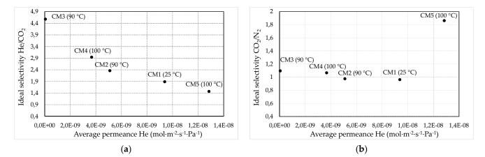
**Figure 9.** Ideal selectivity values of the gas pairs (a)  $He/N_2$  and (b)  $CO_2/N_2$ , with respect to the average values of He permeance for all Carbon/Vycor<sup>®</sup> membranes, that have been acquired over the entire feed pressure range applied.
