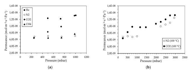
**Figure 8.** Permeance of (**a**) He, N<sub>2</sub>, CO<sub>2</sub>, and CH<sub>4</sub> gases at 100 °C and (**b**) N<sub>2</sub> and CO<sub>2</sub> gases at 100 °C, through the CM5 membrane, as a function of the pressure.
