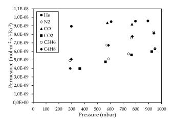
**Figure 2.** Permeance of He, N<sub>2</sub>, CO, CO<sub>2</sub>,  $C_3H_6$ , and  $C_4H_8$  gases through the CM\_1 membrane at 25 °C, with respect to the pressure.
