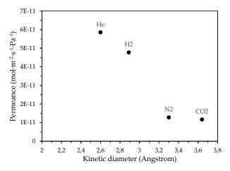
**Figure 6.** Permeance of  $H_2$ , He,  $N_2$ , and  $CO_2$  gases through the CM\_3 membrane at 90 °C, with respect to their kinetic diameter.
