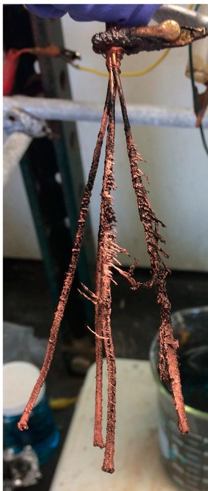
**Figure S7.** Copper wire cathodes with hard coatings (Cu-SWCNT) before rinsing, and drying.
