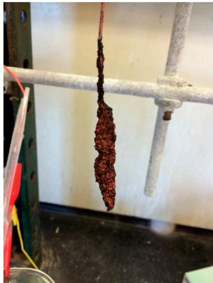
**Figure S4.** Photographic image of Cu-SWCNT composite deposited on the surface of the copper cathode after electrolysis using constant voltage (14 V) power supply:  $[\text{Cu}^{2+}] = \sim 0.095 \text{ M}$ ,  $[\text{SWCNT}] = 2.3 \text{ wt\%}$ .
