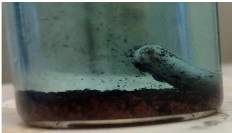
**Figure S1.** Image showing the association of the aggregates with the magnetic stir bar indicating the presence of the SWCNTs containing iron catalyst impurities.
