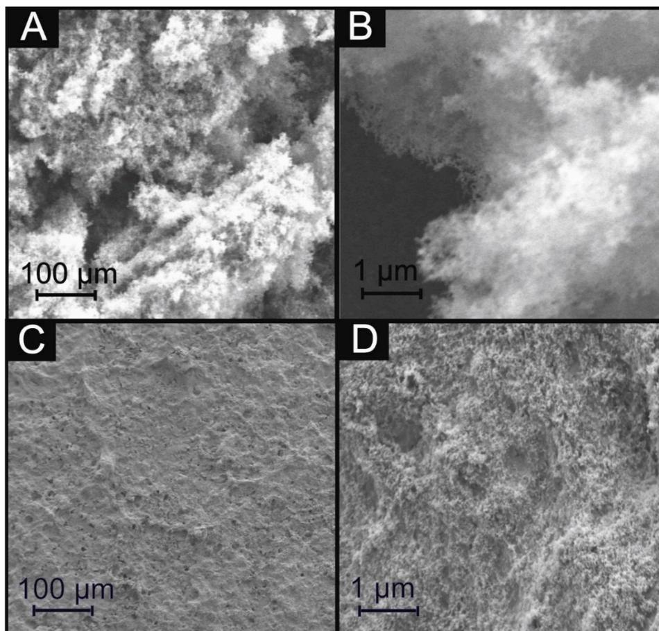
**Figure S2.** SEM images of the graphene@SiC nanocomposite (A,B) and 5 μg graphene@SiC/SPE (C,D) at magnifications of ×250 and ×20 k, respectively.
