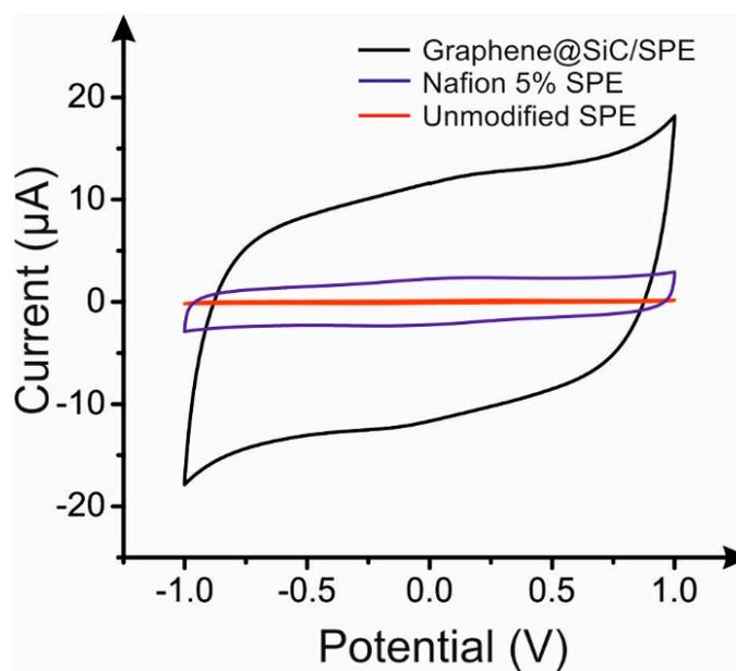
**Figure S3.** Cyclic voltammograms within a 0.1 M H<sub>2</sub>SO<sub>4</sub> utilising a graphene@SiC/SPE, Nafion 5% SPE, and unmodified SPE. Scan rate: 50 mV·s<sup>-1</sup>.
