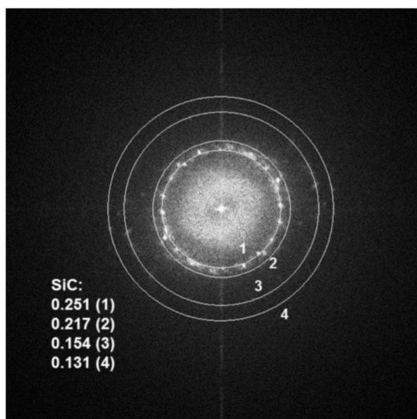
Figure S1. Electron diffraction image of n-SiC core in graphene@SiC.
