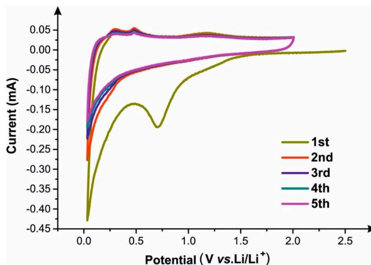
**Figure S4.** Cyclic voltammograms (vs. Li/Li<sup>+</sup>) of the graphene@SiC nanomaterial within a Li-ion cell. Scan rate: 0.1 mV·s<sup>-1</sup>.
