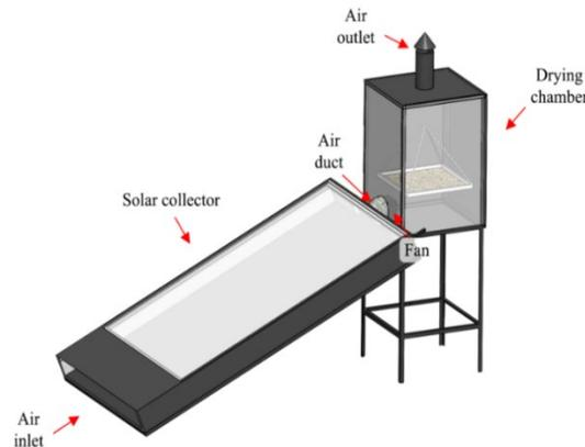
**Figure 2.** Coffee dryer with forced convection.
