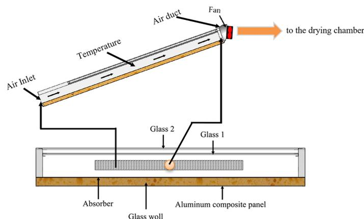
**Figure 1.** Component arrangement of solar coffee dryer equipment.
