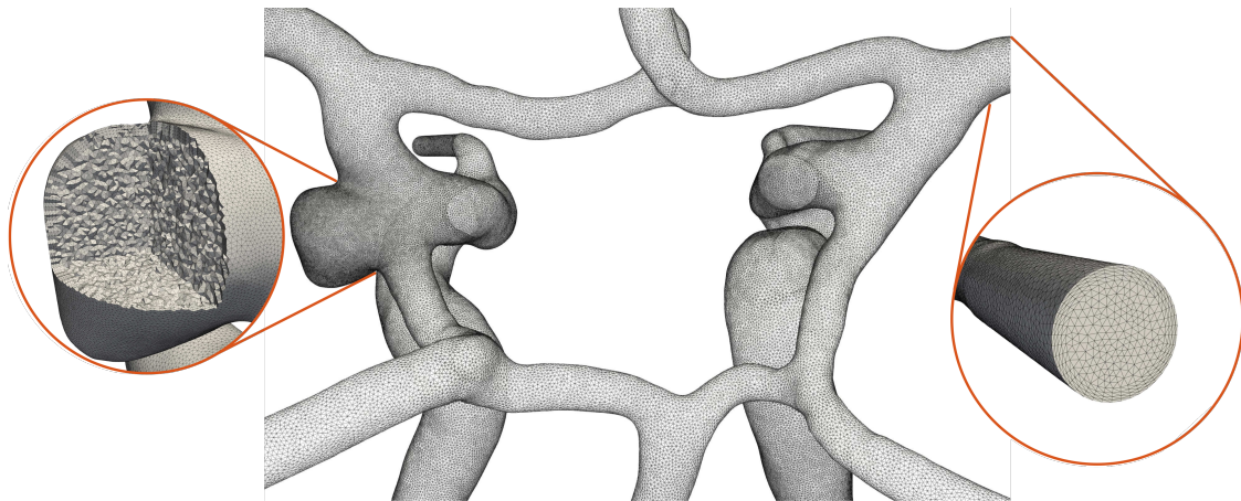
Figure 3. Visualization of the CoW of patient A with highlighted mesh features (orange circles) showing the linear isotropic refinement (left) and structured tetrahedral boundary layers (right).
