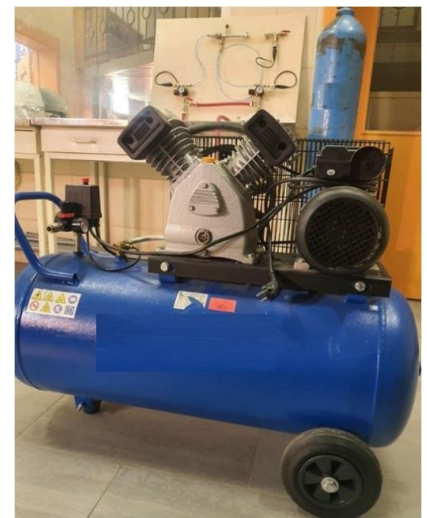
Figure 2. A sketch (a) and an exterior (b) of the test bench [compiled by the authors Y.V. Martynenko, V.I. Bolobov]: 1—compressor; 2—receiver; 3—pressure gauge at receiver; 4, 8—ball valve; 5—reducer; 6—pressure transmitter; 7—compressed air supply line; 9—constrictor nozzle; 10—programmable logic controller; 11—personal computer.
