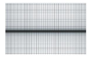
Figure 4. Mesh used in CFD calculations.
