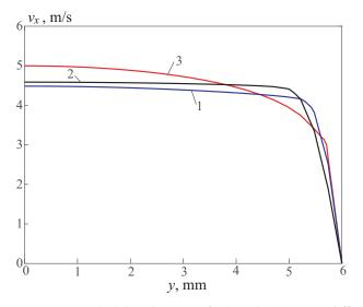
**Figure 10.** Radial distributions of oil axial velocity in different pipeline cross sections at x = 0.5 m (line 1), x = 1.5 m (line 2), and in the exit section (line 3).
