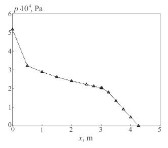
Figure 13. Distribution of cross-section averaged oil pressure.
