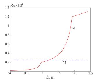
**Figure 9.** Distributions of oil Reynolds numbers along length. Line 1 corresponds to the numerical calculation at variable viscosity, and line 2 corresponds to the theoretical calculation.
