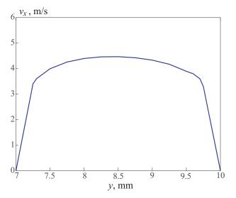
Figure 11. Radial distribution of the axial water velocity in the outlet section.
