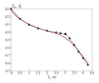
**Figure 7.** Mass–average water temperature distributions along the length. The solid line corresponds to the results obtained on the basis of the theoretical approach, and the dotted line with triangular marks corresponds to the results of numerical calculations.
