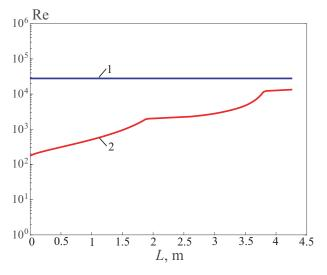
**Figure 8.** Distributions of Reynolds numbers obtained in a theoretical calculation. Line 1 corresponds to water, and line 2 corresponds to oil.
