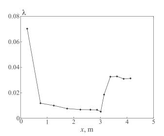
Figure 14. Distribution of the coefficient of friction along the length of the pipe.
