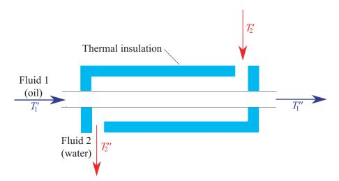
Figure 2. Scheme of counterflow heat exchanger.
