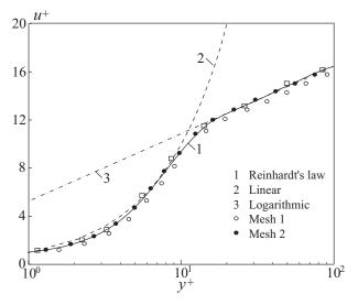
Figure 3. Velocity profiles in the boundary layer.
