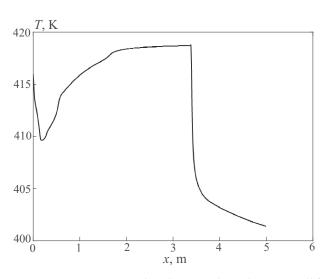
Figure 12. Temperature distributions along the pipe wall from the oil side.
