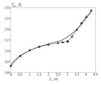
**Figure 6.** Distributions of the mass average temperature of oil along the length. The solid line corresponds to the results obtained on the basis of the theoretical approach, and the dotted line with triangular marks corresponds to the results of numerical calculations.
