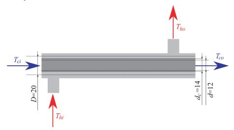
Figure 5. Scheme of parallel flow heat exchanger (dimensions are provided in millimetres).
