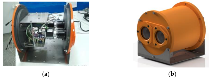
Figure 3. Underwater TSS: (a) Inner module part; (b) Underwater technical stereo vision system.
