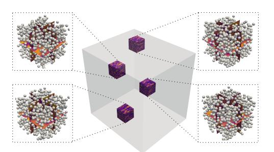
**Figure 28.** Flow visualization in multiple sub-domains at the steady state. The streamlines and rigid spheres for each sub-domain are shown in the sub-images.
