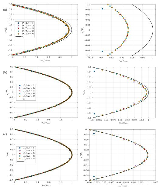
of the profiles corresponding to  $D_c/\Delta x = 6$ , 12 and 24 with respect to the analytical solution  $u_s$  can be easily noticed, this difference is insignificant for  $D_c/\Delta x = 48$  and 96.
