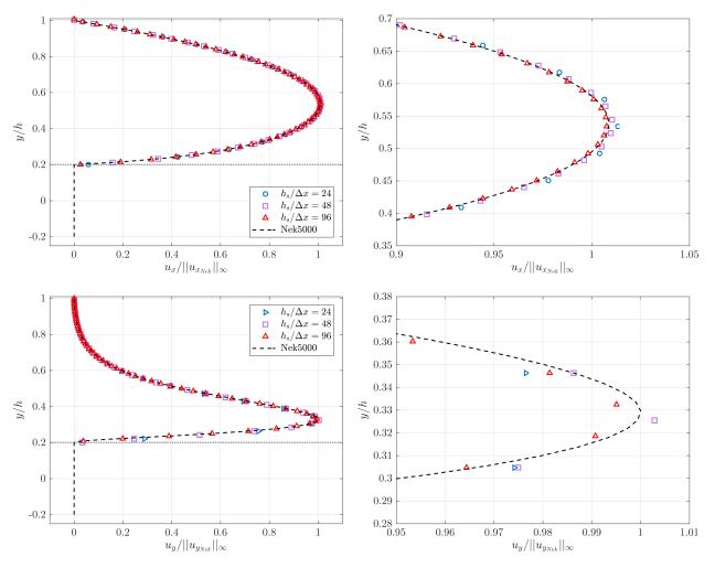
**Figure 16.** Profiles of  $u_x$ ,  $u_y$  and  $u_z$  for  $h/\Delta x = 24, 48, 96$  along the wall-normal direction, profile set at  $(x_1, z_1)$ .
