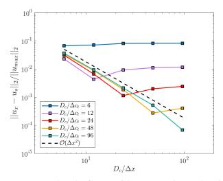
**Figure 9.** Combined influence of the ratios  $D_c/\Delta c_t$  and  $D_c/\Delta x$  on the convergence of the method.
