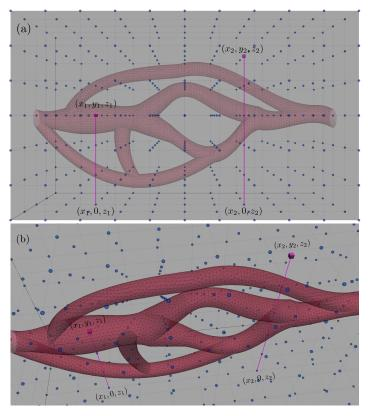
**Figure 3.** Ray-tracing approach employed for two nodes located at  $(x_1, y_1, z_1)$  and  $(x_2, y_2, z_2)$ : (a) front and (b) top-left views of the blood vessel.
