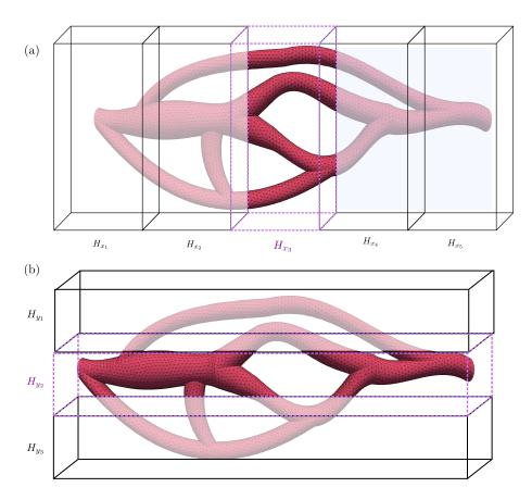
**Figure 5.** (a) Subdivision of the computational domain along *y* into 5 subdivisions:  $H_{x_1}, \ldots, H_{x_5}$ . If a node belongs to  $H_{x_3}$ , the loop over the set of triangles is reduced to the triangles belonging to  $H_{x_3}$ . (b) Subdivision of the computational domain along *x* into 3 subdivisions:  $H_{y_1}, \ldots, H_{y_2}$ . If a node belongs to  $H_{y_2}$ , the loop over the set of triangles is reduced to the triangles belonging to  $H_{y_2}$ .
