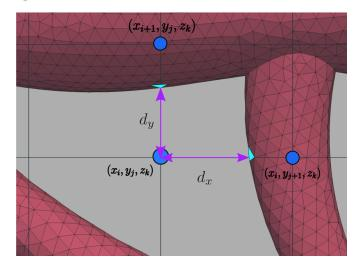
**Figure 4.** Computation of the distances between the grid node and the intersecting triangles in both x and y directions denoted respectively  $d_x$  and  $d_y$ .
