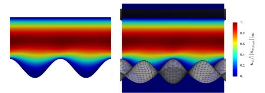
**Figure 11.** Contours of  $u_x/||u_{x_{Nek}}||_{\infty}$  at the steady state on a plane located at z = 1.19 orthogonal to the *z* axis. Left: Nek5000, right: Direction Splitting,  $h_s/\Delta x = 96$ .
