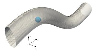
Figure 23. STL triangulation of the pipe wall used in the simulations.
