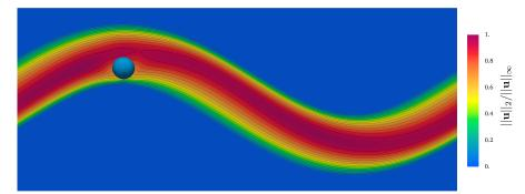
**Figure 24.** Snapshot of  $||\mathbf{u}||_2/||\mathbf{u}||_{\infty}$  for Re = 115 and  $(x_p/R_c, y_p/R_c, z_p/R_c) = (1, 0.5, 0)$  as the initial position of the particle in the pipe.
