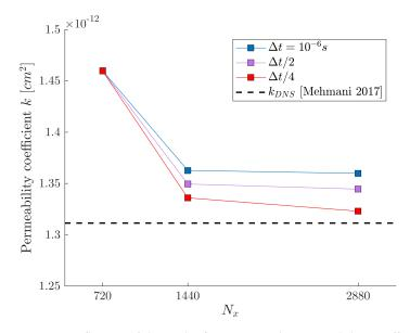
Figure 22. Influence of the grid refinement on the permeability coefficient *k*.
