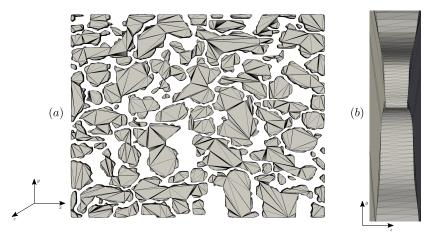
**Figure 19.** STL triangulation of the sandstone rock used in the simulations: (a) xy view and (b) yz view showing a single triangle in the *z* direction.
