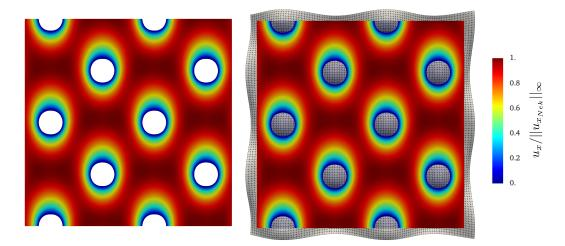
**Figure 13.** Contours of  $u_x / ||u_{x_{Nek}}||_{\infty}$  at the steady state on a plane located at y = 0.15 orthogonal to the *y* axis. Left: Nek5000, right: Direction Splitting,  $h_s / \Delta x = 96$ .
