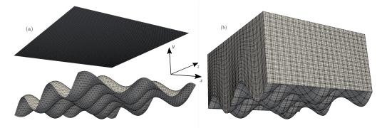
**Figure 10.** (**a**) STL triangulation corresponding to the semi-wavy configuration in *x* and *y* directions considered for the simulations, (**b**) computational domain used in Nek5000.
