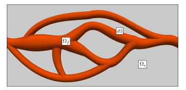
**Figure 1.** Definition of the current framework. The fluid domain and the solid domain are defined by  $\Omega_f$  and  $\Omega_s$ , respectively.  $d\Omega$  denotes the fluid-solid interface.
