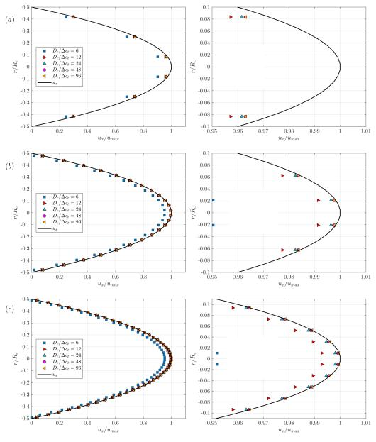
an axisymmetric cylinder. The results associated to  $D_c/\Delta x = 96$  are not showed here but an excellent agreement with the solution is obtained, except for  $D_c/\Delta c_t = 6$ .
