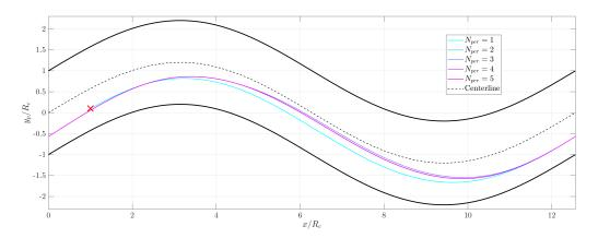
**Figure 26.** Trajectory of the particle in the *xy* plane, sequenced as periods (colored lines), case Re = 113. The red cross indicates the initial particle position, the bold black lines correspond to the pipe interface, and the dashed black line correspond to the centerline of the pipe.
