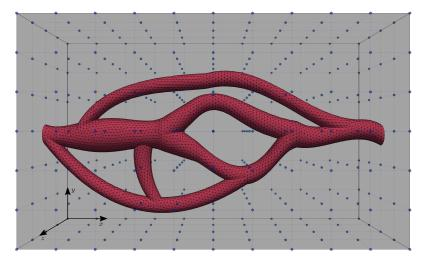
**Figure 2.** STL file of a blood vessel positioned in a cuboid computational domain. The blue dots correspond to the field (i.e.,  $u_x$ ,  $u_y$ ,  $u_z$ , p) nodes.
