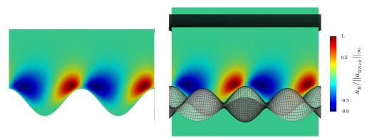
**Figure 12.** Contours of  $u_y/||u_{y_{Nek}}||_{\infty}$  at the steady state on a plane located at y = 0.19 orthogonal to the *z* axis. Left: Nek5000, right: Direction Splitting,  $h_s/\Delta x = 96$ .
