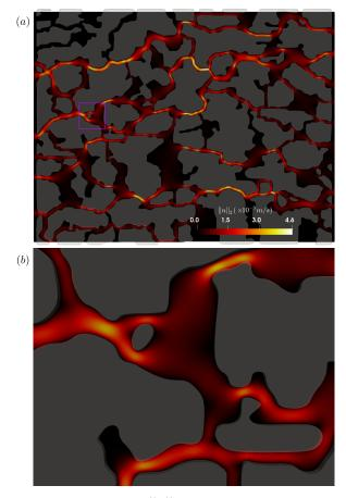
**Figure 21.** Contours of  $||\mathbf{u}||_2$  (in m/s) at the steady state. The STL triangulation is also shown here in light gray. (a) Whole computational domain, (b) zoomed view of the purple square as shown in (a).
