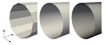
**Figure 6.** STL triangulations of the pipe wall, left to right:  $D_c / \Delta c_t = 6,24$  and 96.
