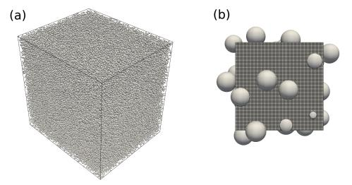
**Figure 27.** (**a**) Computational domain showing all rigid spheres. (**b**) Sub-domain on a single computing core showing well-resolved spheres with a grid resolution of 24 grid points per diameter.
