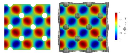
**Figure 14.** Contours of  $u_z/||u_{z_{Nek}}||_{\infty}$  at the steady state on a plane located at y = 0.15 orthogonal to the *y* axis. Left: Nek5000, right: Direction Splitting,  $h_s/\Delta x = 96$ .
