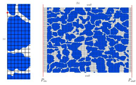
**Figure 20.** Sketch of the flow configuration: (**a**) upstream part of the domain without any buffer region and (**b**) full domain with inlet and outlet buffer regions and a thin layer removed in the *y* direction.
