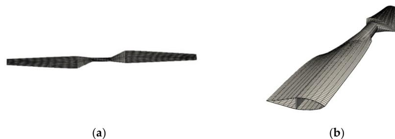
**Figure 3.** The mesh generated for the solid blade, which includes the D-cap and trailing edge with the 29,446 structural mesh cells in number: (a) Blade solid mesh; (b) Blade solid mesh internal structure.
