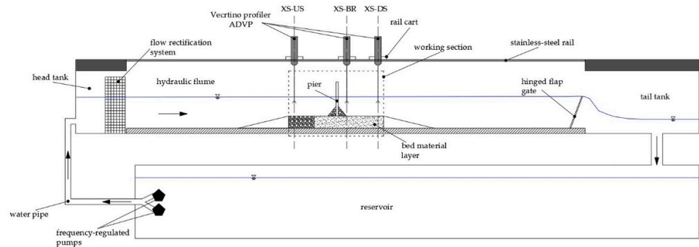
**Figure 2.** Scheme of the hydraulic flume setup.
