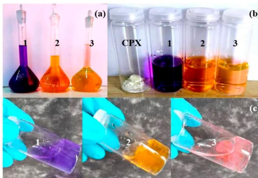
**Figure 7.** Adsorption tests of CPX hydrogel: (1) gentian violet; (2) methyl orange; (3) eosin; (a) stock solution; (b) initial time; (c) after 24 h [97].
