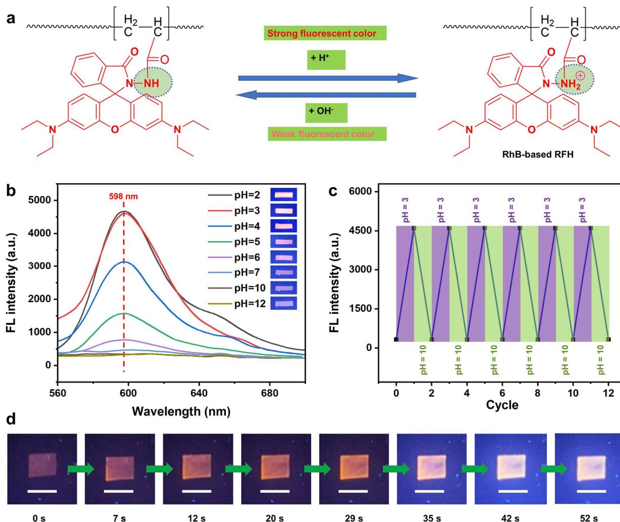
**Figure 3.** (a) The mechanism of pH-responsive fluorescent color-changing performance of the RFH. (b) The pH-dependent fluorescent emission spectra of RFH ( $\lambda_{\text{exc}} = 365 \text{ nm}$ ). (c) The six cycles between pH = 3 and 10 buffer solution of the RFH. (d) The color-changing process of the RFH from pH = 10 to 3.
