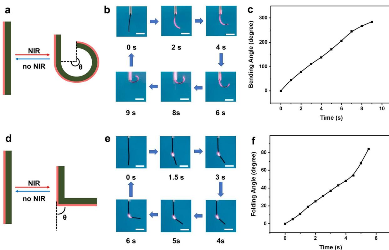
**Figure 5.** (a–c) The bending process of the bi-layer hydrogel actuator under  $7.5 \text{ W/cm}^2$  of NIR light irradiation. (d–f) The folding process of the bi-layer hydrogel actuator under  $60 \text{ W/cm}^2$  of NIR light irradiation. All scale bars are 5 mm.
