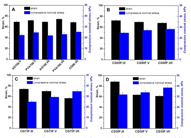
**Figure 2.** Maximum sustained compression (black color) and compressive strength (blue color): (**A**) control samples; (**B**) composite hydrogels prepared with a weight ratio between XG and PVA of 9:1; (**C**) composite hydrogels prepared with a weight ratio between XG and PVA of 3:1; (**D**) composite hydrogels prepared with a weight ratio between XG and PVA of 1:1. All the data were expressed as the mean of three individual measurements  $\pm$  SD. The SD is presented as error bars.
