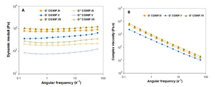
**Figure 11.** Effect of the cryogenic cycles number (III, V and VII) on the variation of (**A**) storage modulus (G') (*solid symbols*) and loss modulus (G") (*open symbols*), (**B**) complex dynamic viscosity ( $|\eta^*|$ ) function of angular oscillation frequency at 25 °C for XG-based composite hydrogels obtained with a weight ratio between XG and PVA of 9:1, and Feteasca Neagra polyphenolic extracts.
