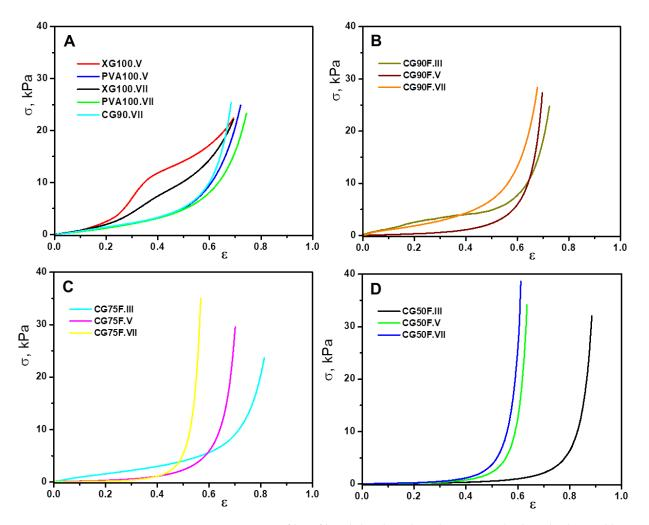
**Figure 1.** Stress-strain profiles of lyophilized XG-based composite hydrogels obtained by uniaxial compression using a cross-head speed of 0.2 mm min<sup>-1</sup> and a force of 20 N: (**A**) control samples; (**B**) composite hydrogels prepared with a weight ratio between XG and PVA of 9:1; (**C**) composite hydrogels prepared with a weight ratio between XG and PVA of 3:1; (**D**) composite hydrogels prepared with a weight ratio between XG and PVA of 1:1.
