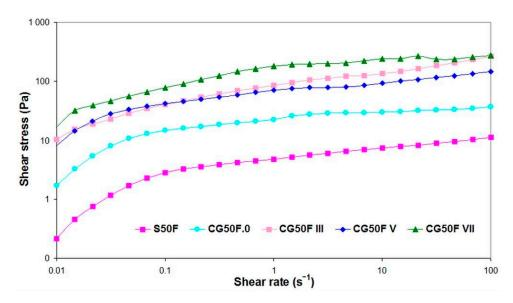
**Figure 8.** Rheograms (shear stress vs. shear rate) recorded for XG-based composite hydrogels obtained with a weight ratio between XG and PVA of 1:1, and Feteasca Neagra polyphenolic extracts in initial state, lyophilized and cryogenated at different cryogenic cycles.
