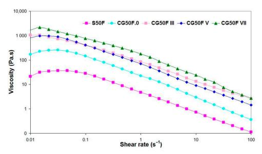
**Figure 7.** Viscosity as a function of shear rate for XG-based composite hydrogels obtained with a weight ratio between XG and PVA of 1:1, and Feteasca Neagra polyphenolic extracts in initial state, lyophilized or cryogenated at different cryogenic cycles.
