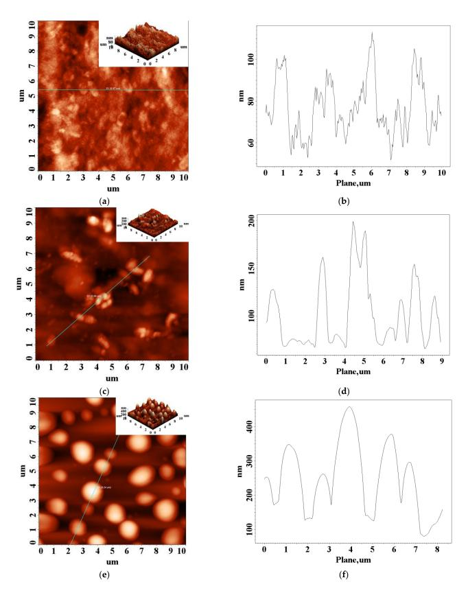
**Figure 6.** Height-contrast AFM 2D images (3D images as inset) and profiles along the straight line: (**a**,**b**): XG100.VII; (**c**,**d**): XG90PVA.III, and (**e**,**f**): XG50PVA.III.
