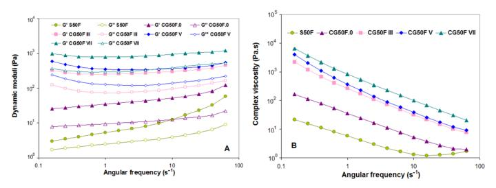
**Figure 9.** Effect of the lyophilization and cryogenic cycles number (III, V and VII) on the variation of (**A**) storage modulus (G') (solid symbols) and loss modulus (G'') (open symbols) and (**B**) complex dynamic viscosity ( $|\eta^*|$ ) function of angular oscillation frequency at 25 °C for XG-based composite hydrogels obtained with a weight ratio between XG and PVA of 1:1, and Feteasca Neagra polyphenolic extracts.
