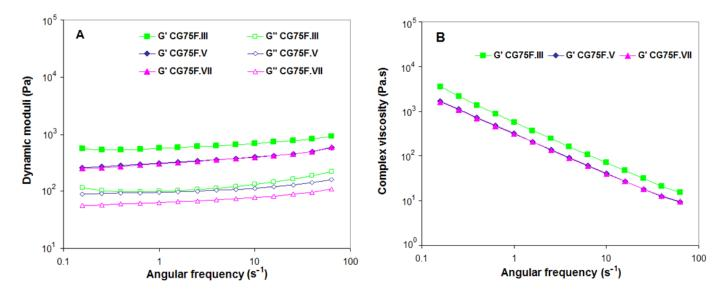
**Figure 10.** Effect of the cryogenic cycles number (III, V and VII) on the variation of (**A**) storage modulus (G') (*solid symbols*) and loss modulus (G") (*open symbols*), (**B**) complex dynamic viscosity ( $|\eta^*|$ ) function of angular oscillation frequency at 25 °C for XG-based composite hydrogels obtained with a weight ratio between XG and PVA of 3:1, and Feteasca Neagra polyphenolic extracts.
