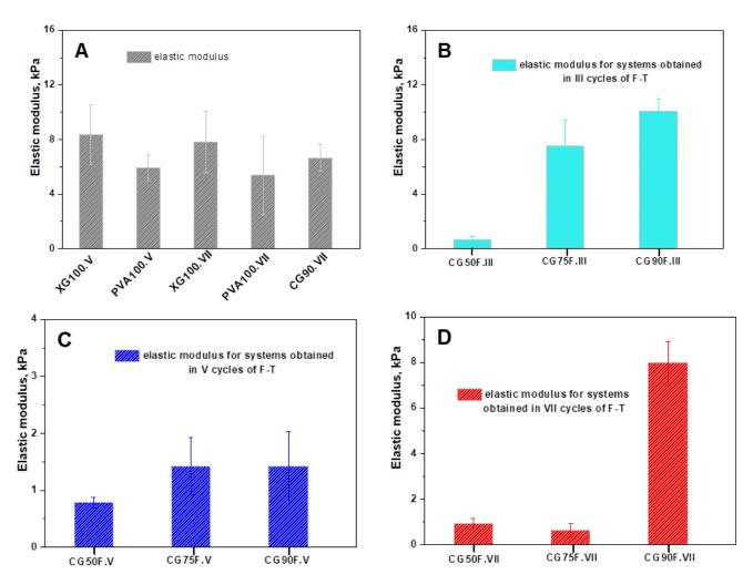
**Figure 3.** Elastic modulus of the polyphenol-loaded XG/PVA composite hydrogels: (**A**) control samples; (**B**) composite hydrogels prepared in III cycles of F-T; (**C**) composite hydrogels prepared in V cycles of F-T; (**D**) composite hydrogels prepared in VII cycles of F-TAll the data were expressed as the mean of three individual measurements  $\pm$  SD.
