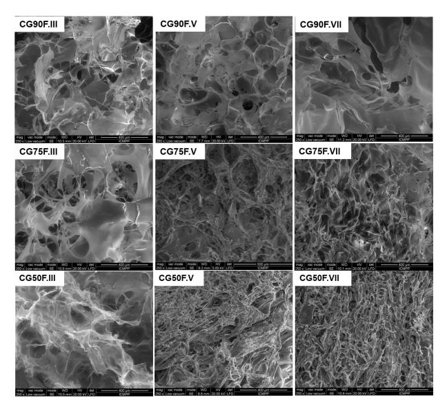
Figure 4. SEM micrographs of the lyophilized XG-based composite hydrogels.
