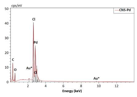
Figure 2. EDS absorption spectrum of CNS-Pd.
