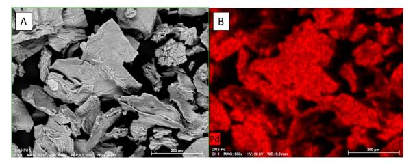
**Figure 1.** SEM images of CNS-Pd (**A**) and distribution of Pd on the catalyst's surface, obtained with EDS (**B**).
