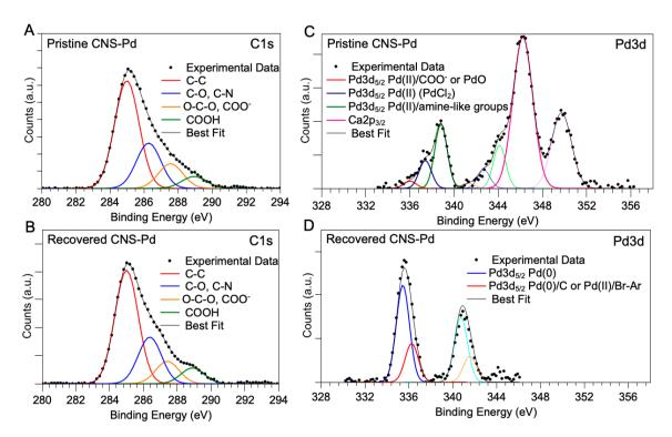
**Figure 3. (A)** XPS C 1s core-level spectra acquired on pristine CNS and **(B)** CNS recovered after catalysis; **(C)** XPS Pd 3d core-level spectra acquired on CNS before and **(D)** after catalysis.
