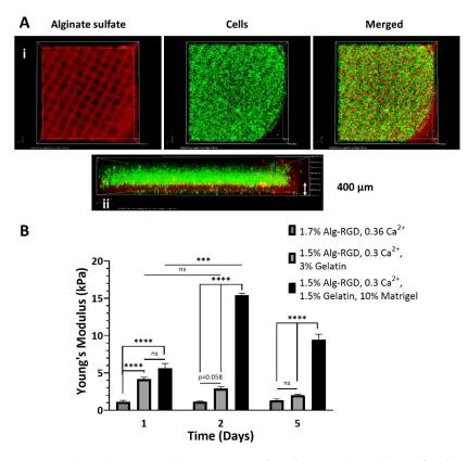
**Figure 5.** Three-dimensional bio-printing of cardiac patches. (**A**) Confocal images of XY (i) and reconstructed YZ (ii) planes of the two-compartment, 3D bio-printed cardiac patch. Red—Alginate sulfate; Green—fluorescently labeled cells. (**B**) Young's modulus of 3D bio-printed cardiac patches over time, using different core bioink. Data are mean  $\pm$  SEM, n = 3–4, \*\*\* *p* < 0.001, \*\*\*\* *p* < 0.0001, Tukey's test, two-way ANOVA.
