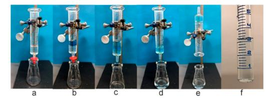
Figure 13. Gel column for the dye absorption experiment. (a) Gel column before the experiment; (b) Gel column after loading with 1 mL of 32.7  $\mu$ M TBO stock solution; (c) Washing the column with 1 mL of DI water; (d) Gel column at the end of the experiment; (e) Inverted gel column after the completion of the experiment; (f) Very light blue aqueous solution collected from the gel column.
