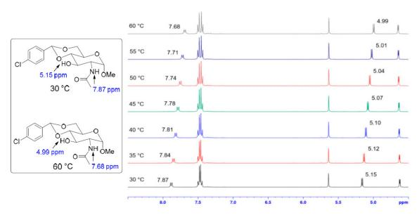
**Figure 6.** Stacked <sup>1</sup>H-NMR (400 MHz) spectra of compound **3** at temperature 30–60 °C. The sample was prepared at 12.5 mg/mL in DMSO-d<sub>6</sub>.
