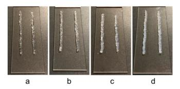
**Figure 9.** Extruded gels formed by compounds **11** (a,b) and **13** (c,d) in DMSO/H<sub>2</sub>O (1:1). The concentrations of the gels are 5.0 mg/mL for (a,c); 10.0 mg/mL for (b,d).
