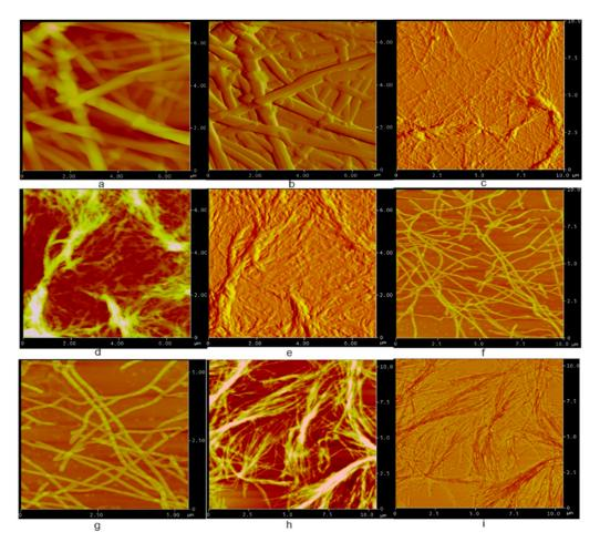
**Figure 5.** AFM images of the gels formed by gelators **11–13**, (**a**,**d**,**f**,**g**,**h**) are height images, and the rest are phase images. (**a**,**b**) **11** in DMSO/H<sub>2</sub>O (v/v 1:2) at 2.0 mg/mL; (**c**-**e**) **12** in EtOH/H<sub>2</sub>O (v/v 1:1) at 2.0 mg/mL; (**f**,**g**) **13** in DMSO/H<sub>2</sub>O (v/v 1:1) at 1.0 mg/mL; (**h**,**i**) **13** in EtOH/H<sub>2</sub>O (v/v 1:1) at 1.0 mg/mL.
