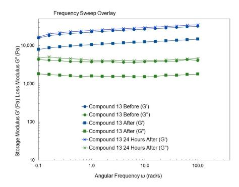
**Figure 11.** Rheology properties (frequency sweep, 0.5% strain) of a gel of compound **13** in DMSO/H<sub>2</sub>O 1:1 at 5 mg/mL before and after extrusion, and 24 h after extrusion.
