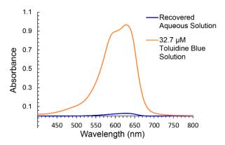
Figure 14. The UV-Vis spectra of the 32.7  $\mu$ M TBO solution loaded to the top of the gel in Figure 13b and the liquid collected from the gel column (Figure 13f). The TBO was almost fully absorbed by the gel.
