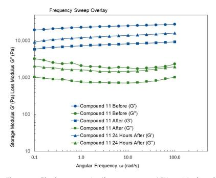
**Figure 10.** Rheology properties (frequency sweep, 0.5% strain) of a gel of compound **11** in DMSO/H<sub>2</sub>O 1:1 at 5 mg/mL before and after extrusion, and 24 h after extrusion.
