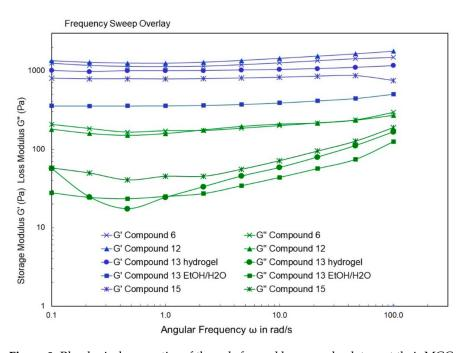
**Figure 8.** Rheological properties of the gels formed by several gelators at their MGCs: compound **6** in EtOH/H<sub>2</sub>O (1:1) at 0.74 mg/mL; compound **12** in EtOH/H<sub>2</sub>O (1:1) at 0.67 mg/mL, compound **13** in water at 0.36 mg/mL and in EtOH/H<sub>2</sub>O (1:2) at 0.36 mg/mL and compound **15** in DMSO/H<sub>2</sub>O (1:1) at 0.71 mg/mL. All frequency sweeps were using 0.1% strain.
