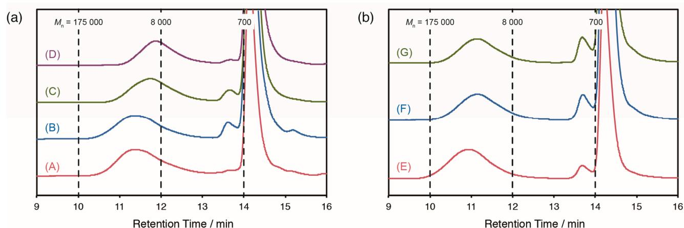
**Figure S2.** GPC curves of reaction mixtures after polymerization using AIBN (a) and a redox system (b) as an initiator: entries 1 (A), 2 (B), 3 (C), 4 (D), 9 (E), 10 (F), and 11 (G).
