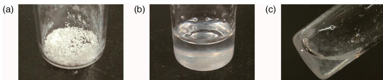
**Figure S1.** Photographs of cross-linked polymer **2** after purified (a) and swollen with anisole (b, c).
