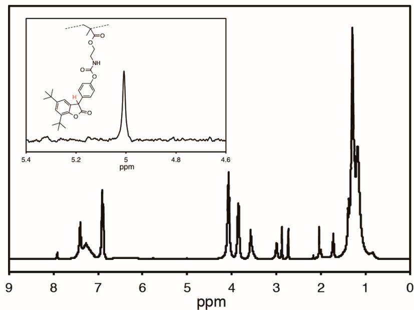
**Figure S3.**  $^1\text{H}$  NMR spectrum of a reaction mixture after de-cross-linking of **5**. The insert shows a spectrum magnified. The conversions of cross-linking were calculated from the peak at 5 ppm, which originates from unreacted ABF units in **5**.
