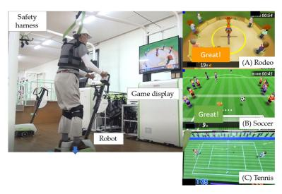
**Figure 2.** The balance exercise assist robot (BEAR) system. The BEAR moves backwards and forwards, as well as left and right, according to shifts in the operator's center of gravity. These movements can be incorporated into balance exercises by playing three video games: (**A**) rodeo; (**B**) soccer; and (**C**) tennis.
