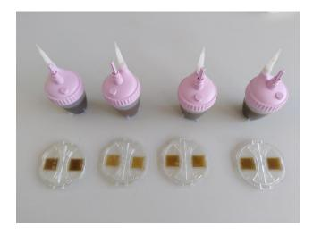
Figure 2. Mini-FLOTAC and Fill-FLOTAC devices used for quantitative coprology (original).
