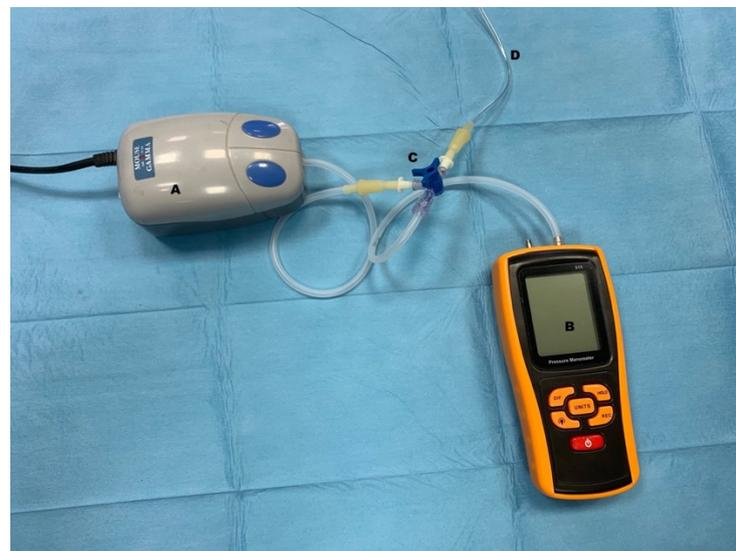
**Figure 3.** Image of instrumentation used for burst pressure (BP) test. (A) air pump; (B) manometer; (C) three-way stopcock; (D) tube to the construct.
