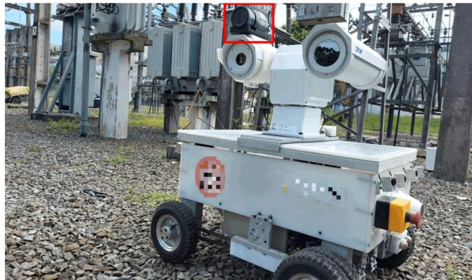
**Figure 4.** A photo of our AGV equipped with the FLIR A700 (marked with the red box) and the FLIR A310 (the white one, with two separate lenses) cameras in a substation floor. The A310 was not used to take any photos for this dataset, but was used for pan-tilt purposes for other mounted cameras.
