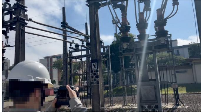
**Figure 3.** A technician capturing images using the FLIR T540 camera.
