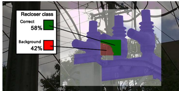
**Figure 9.** Example of how Box<sup>i</sup> is ill-suited for the recloser object class, with the ground truth outlining the object in purple. In this case, of the 20% innermost portion of the white box that should identify the object class, 42% of the total area is actually background, represented here in red.
