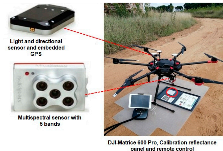
Figure 2. Multi-rotor DJI-Matrice 600 and the MicaSense RedEdge-MX sensor used in the study. “Light and directional sensor” refers to the Downwelling Light Sensor (DLS).
