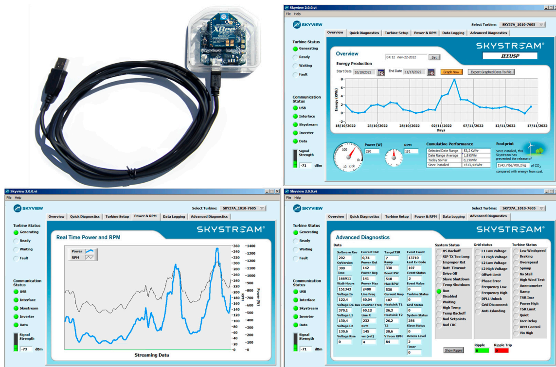
Figure 8. SWT's monitoring system components: wireless PC adapter 2.4 GHZ and screen captures of the monitoring software Skyview®.
