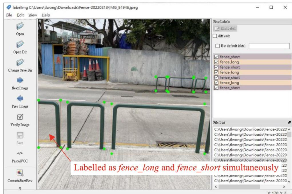
**Figure 5.** Example of labelling partially out-of-view objects. A partially out-of-view object was labelled as *fence\_long* and *fence\_short* simultaneously since it cannot be classified by a single image.
