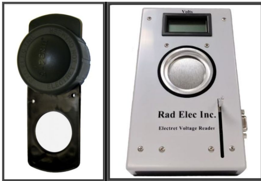
Figure 4. The LLT-OO Chamber passive radon detector (L), and the Rad Electret reader (R).
