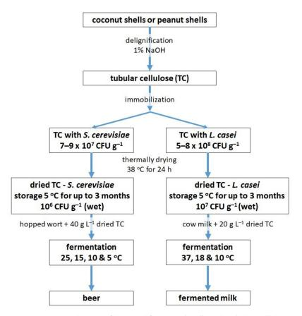
Figure 1. The production of beer and fermented milk with tubular cellulose.
