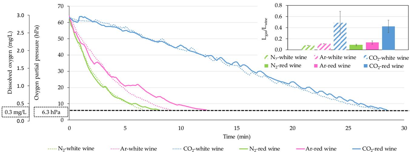
**Figure 3.** Kinetics of oxygen removal by sparging with N<sub>2</sub>, CO<sub>2</sub>, and Ar in a volume of 2.5 L of white and red wine. Average of three repetitions were performed with each gas.
