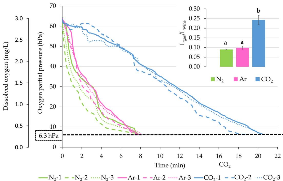
**Figure 1.** Kinetics of oxygen removal in model wine with the different inerting gases tested. Average of three repetitions were performed with each gas. Different letter in the bar graph indicated statistically significant differences.
