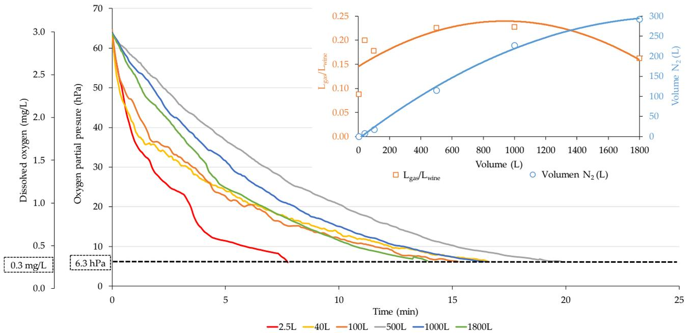
**Figure 2.** Kinetics of oxygen removal by sparging with N<sub>2</sub> in different volumes of model wine. Average of three repetitions were performed with each gas.
