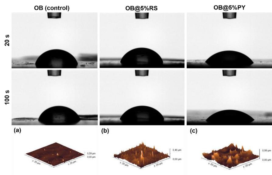
**Figure 7.** Contact angles of a water droplet (initial volume of 8 μL) deposited onto different composite surfaces (OB, OB@5%RS and OB@5%PY) after 20 and 100 s post deposition. AFM micrographs (20 μm × 20 μm) of the different composite surfaces (a) OB, (b) OB@5%RS and (c) OB@5%PY.
