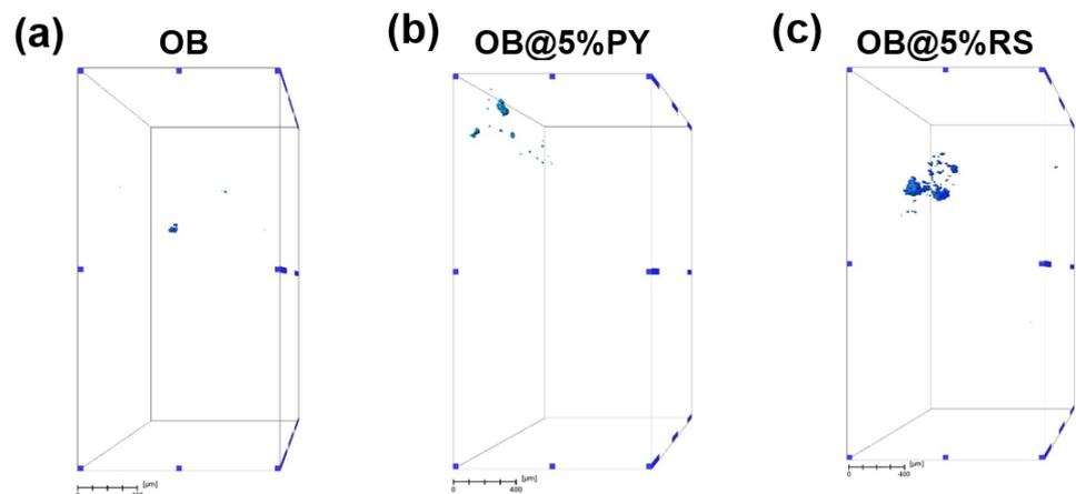
**Figure 9.** Micro-computed X-ray tomography analysis (scale bar of  $400\ \mu\text{m}$ ). Volume rendering of the segmented pores in (a) OB (unmodified sealer); (b) OB@5%PY (sealer doped with 5%PY); and (c) OB@5%RS (sealer doped with 5%RS).
