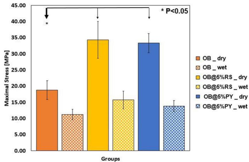
**Figure 8.** Evolution of maximal stress under compression for OB, OB@5%RS and OB@5%PY in dry conditions; and after immersion in water for 72 h. \*  $p < 0.05$  bold arrow.
