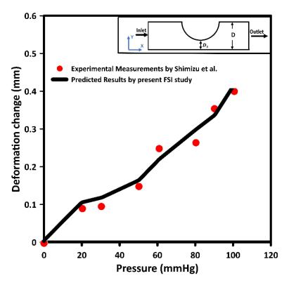
**Figure 3.** Validation of current calculated deformation changes with those of Shimizu et al. [47] at the narrowest segment of a stenotic model.
