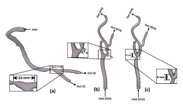
**Figure 1.** Physical model schematic diagram: (a) stenotic RCA—model A, (b) stenotic ICA—model B, and (c) stenotic CCA—model C.
