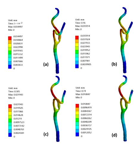
**Figure 11.** CA—model B deformation contours for different times of the cardiac cycle: (a) t = 0.02 s, (b) t = 0.16 s, (c) t = 0.385 s, and (d) t = 0.74 s.
