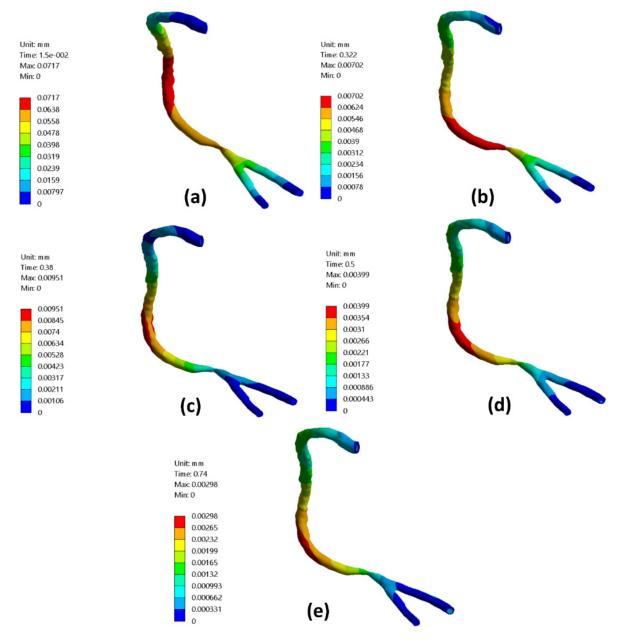
**Figure 10.** RCA—model A deformation contours for different times of the cardiac cycle: (a) t = 0.015 s, (b) t = 0.32 s, (c) t = 0.38 s, (d) t = 0.5 s, and (e) t = 0.74 s.
