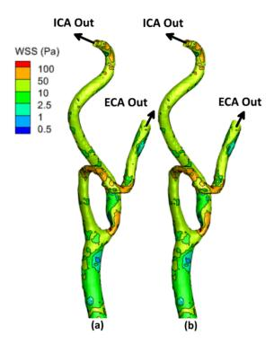
**Figure 5.** WSS contours for stenotic ICA (model B) of the CA at the peak systole of the cardiac cycle: (a) elastic wall, (b) rigid wall.
