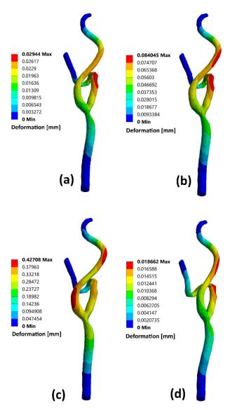
**Figure 12.** CA—model C deformation contours for different times of the cardiac cycle: (a) t = 0.02 s, (b) t = 0.16 s, (c) t = 0.385 s, and (d) t = 0.74 s.
