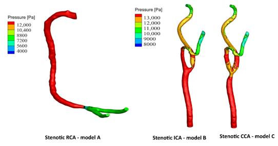
Figure 13. Pressure distribution for the wall compliance models at the peak systole of the cardiac cycle.
