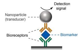
Figure 1. Schematics showing the principle of a typical POC nanobiosensor.
