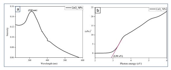
Figure 2. (a) UV-Visible spectrum of CeO<sub>2</sub> NPs, (b) UV-DRS spectrum of CeO<sub>2</sub> NPs.
