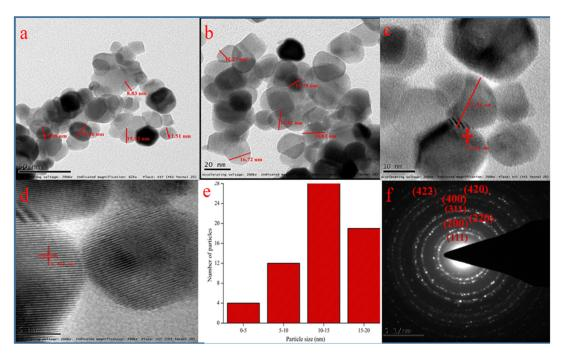
**Figure 4.** TEM images of CeO<sub>2</sub> NPs at different magnifications: (**a**) 50 nm, (**b**) 20 nm, (**c**) 10 nm, (**d**) 5 nm; (**e**) particle size histogram, (**f**) SAED pattern with hkl values.
