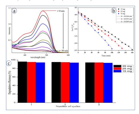
**Figure 6.** (a) UV-Visible absorbance spectra of SY dye during degradation with  $CeO_2$  NPs, (b) kinetic studies of SY dye degradation with  $CeO_2$  NPs, (c) recyclability study of different amounts of catalysts recovered towards degradation of SY Dye.
