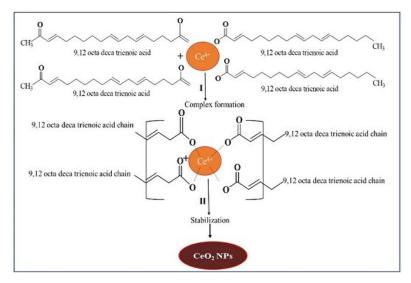
Figure 1. Mechanism of green synthesis of CeO<sub>2</sub> NPs by using E. globulus leaf aqueous extract.
