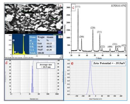
**Figure 3.** (a) SEM image of CeO<sub>2</sub> NPs, (b) EDAX spectrum, (c) XRD diffractogram of synthesized CeO<sub>2</sub> NPs, (d) particle size distribution, and (e) Zeta potential of CeO<sub>2</sub> NPs.
