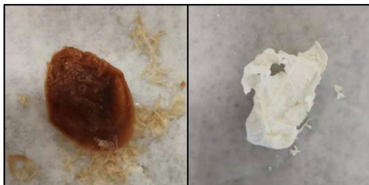
Figure S1. PHA extracted from the mixed microbial consortium grown on acetate. The lyophilized cell pellet is shown left, and the chloroform extracted PHA on the right.
