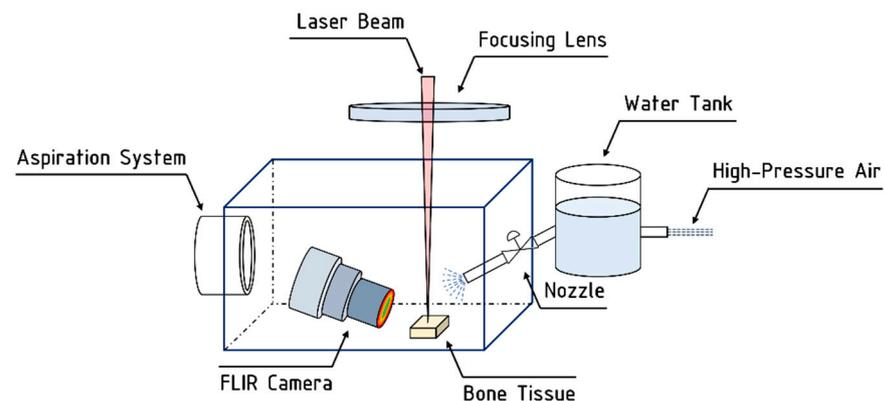
**Figure 2.** Schematic representation of the customized setup employed for laser processing in hybrid air-and-water jet system.
