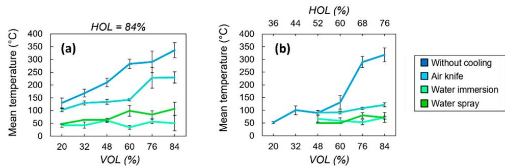
**Figure 8.** Evolution of the mean temperature as a function of the spatial overlaps *VOL* (a) and *HOL* (b) between successive laser pulses for the four different cooling methods. All cavities were ablated with a wavelength of 515 nm at  $P = 6.27$  W and  $RR = 250$  kHz. Error bars represent data standard deviations.
