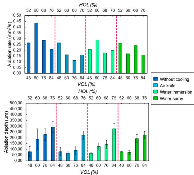
**Figure 9.** Evolution of (top) the ablation rate and (bottom) ablation depth as a function of the spatial overlaps *HOL* and *VOL* between successive laser pulses for the four different cooling methods. All cavities were ablated with a wavelength of 515 nm at  $P = 6.27$  W and  $RR = 250$  kHz.
