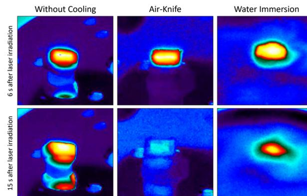
**Figure 7.** Images recorded from IR thermal camera 6 s and 15 s after the start of laser processing in three different processing environments (left: without cooling; center: air-knife; right: water immersion).
