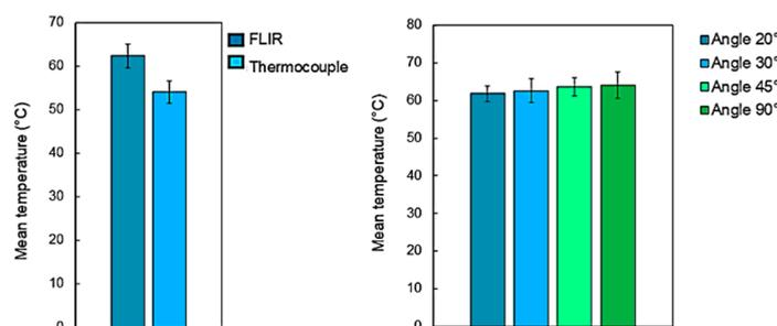
**Figure 3.** (left-hand side) Evolution of the mean temperature of the bone tissue measurement by thermal camera and thermocouples and (right-hand side) influence of the camera's viewing angle on the acquired temperatures. Bone tissue samples were placed on a hot plate kept at a temperature of  $60\text{ }^{\circ}\text{C}$ .
