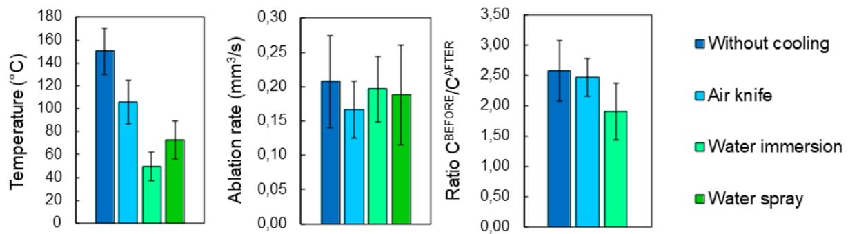
**Figure 6.** Evolution of (left-hand side) the mean temperature, (center) ablation rate and (right-hand side) ratio  $C^{\text{BEFORE}}/C^{\text{AFTER}}$  as a function of cooling environment. For each processing environment, 5 cavities were ablated with a wavelength of 515 nm at  $P = 6.27$  W,  $RR = 250$  kHz and scanning speed  $v = 2500$  mm/s. Error bars represent data standard deviations.
