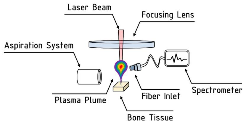
**Figure 4.** Schematic representation of the LIBS setup employed for the analyses.
