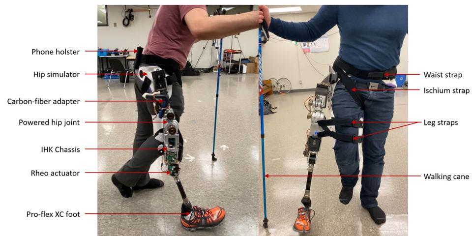
**Figure 7.** Test prosthesis setup attached to hip simulator.
