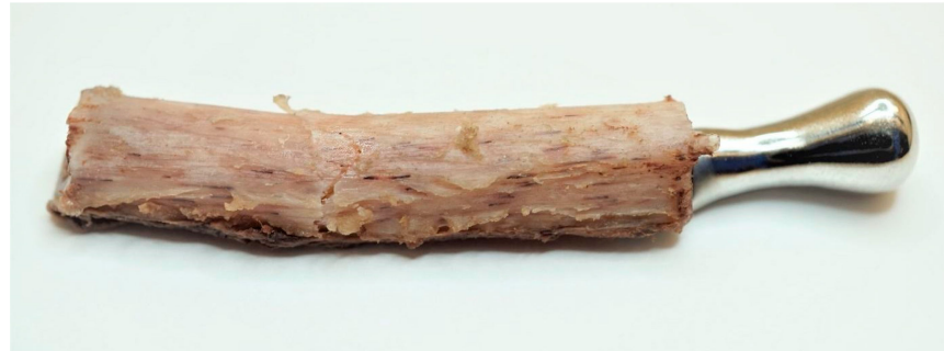
Figure 8. Sample with visible transverse fracture of the bone element.
