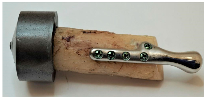
Figure 10. Sample 7, mounted in acrylic resin after testing with no fractures and visible bone displacement from the resin level.
