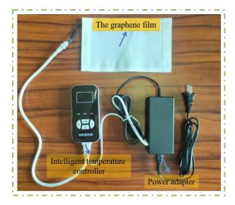
Figure 2. Physical picture of the graphene heating device.
