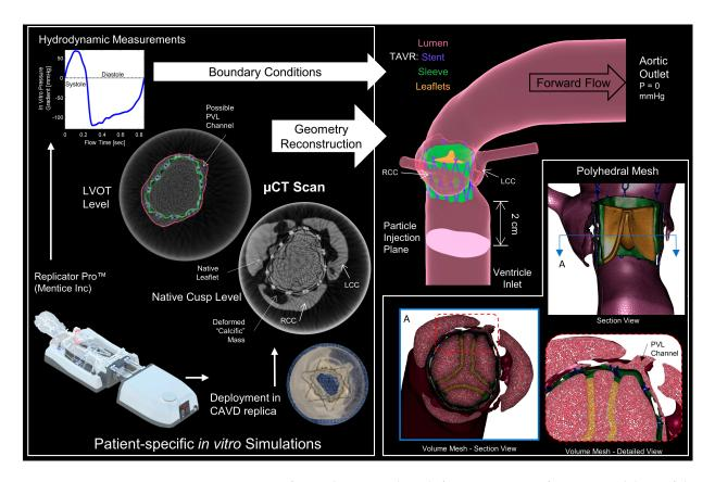
Figure 1. Creation of CFD domain and mesh from  $\mu$ CT scans of in vitro models—Left box—the process of obtaining patient-specific boundary conditions from hydrodynamic studies and segmentation of  $\mu$ CT models (colored to show components). Top right—final sample reconstructed CFD domain. Bottom right box—Polyhedral mesh showing the resolution within the PVL channels and cell volume distinction.
