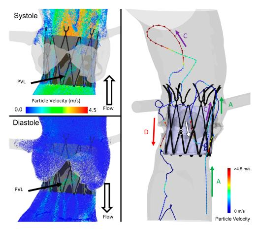
**Figure 3.** Evidence of platelet entering and reentering in both flow phases—Left shows platelets entering the PVL channels of Anatomy A in both systolic phase and diastolic phase. Right shows a pathline of platelet from (**A**) entering the channel in systole, (**B**) reentering in diastole and recirculation for another cycle, (**C**) exiting in 3rd systole into the aorta, and finally (**D**) washing through the PVL channel in the final diastolic phase.
