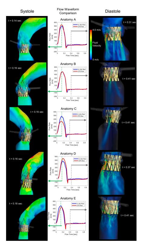
**Figure 2.** Flow pattern and waveform comparison—Volume of fluid (VOF) rendering of the fluid velocity of the CFD solution in systole (**left**) and diastole (**right**). Overlays of the flow waveform, comparing the in vitro and in silico solutions, with systole (green) and diastole (gray) timepoints labeled.
