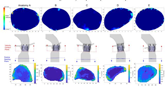
**Figure 6.** Contour plots of LVOT velocity and concentration of platelets entering the PVL domain—Top are velocity contour plots in the LVOT perpendicular to the bottom of the TAVR stent. Bottom contours represent the concentration of the starting position of the PVL platelets in the LVOT, showing concentrations towards the lumen surface. Each column represents the patient-specific anatomies (**A–E**).
