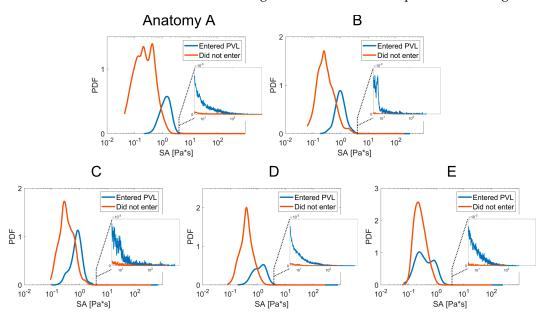
**Figure 5.** Probability density function (PDF) of the platelets stress accumulation (SA) comparison—Showing the increased stress accumulation of platelets entering the PVL channels (blue peaks shifted right). Inset graph highlights higher stress values (>5 Pa  $\times$  s). Each PDF represents the patient-specific anatomies (A–E).
