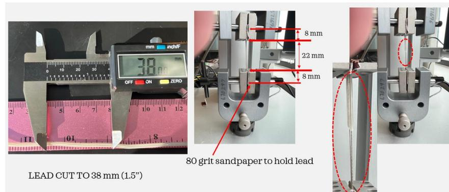
Figure 9. Testing tensile strength of the silicone insulation of the Medtronic extension.
