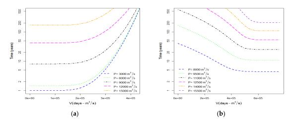
**Figure 7.** (a) Conditional return periods  $T_{(V>v|P\leq p)}$ , (b) Conditional return periods  $T_{(V>v|P>p)}$ .
