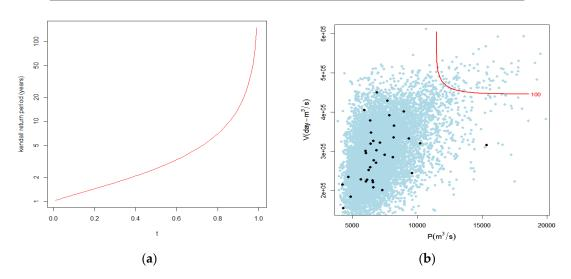
**Figure 8.** (a) The plot between t (levels) and Kendall return period. (b) The contour plot of the peak and volume for the secondary return period over 100 years.
