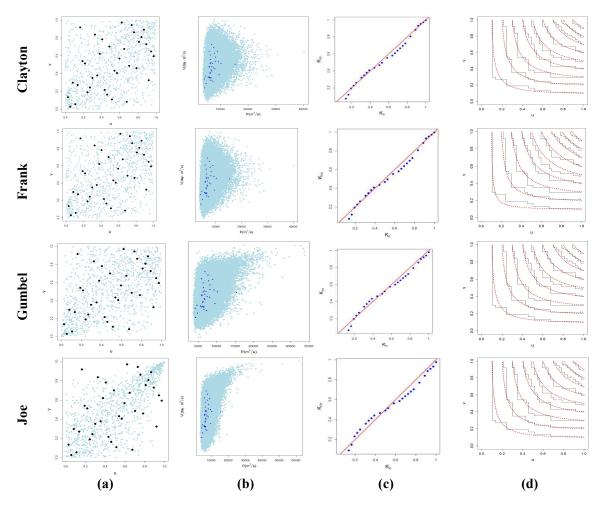
**Figure 4.** (a,b) The comparison of observed data (black dots) and 10,000 random pairs generated data (blue dots) from the copula for peak-flow and volume. (c) The QQ-plot of the copula (Kendall function from the data and the copula). (d) The comparison between empirical and theoretical copula.
